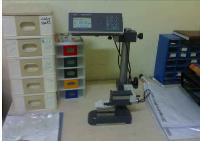
Fig.4. the method of measuring the surface roughness
