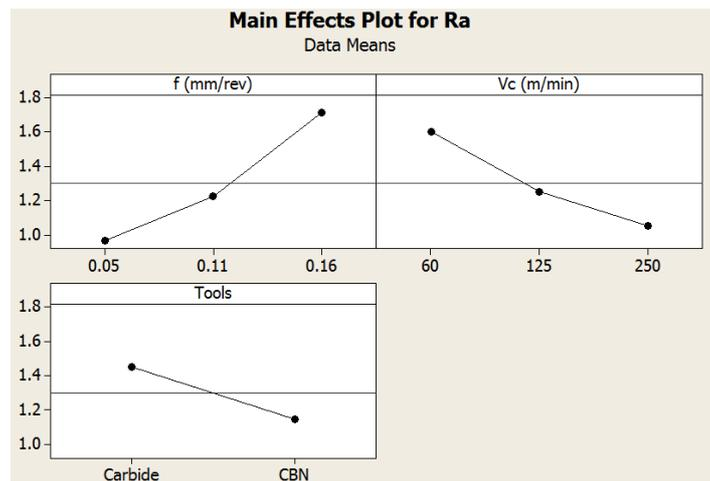
Fig.6 Main effect of parameters on surface roughness
