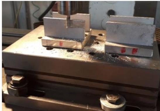
Figure 8. Machining of the Aluminum Workpiece
