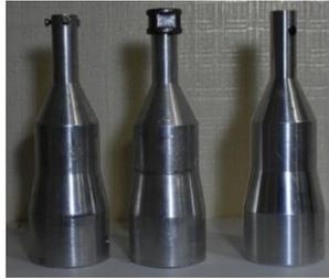
Figure 4. Three separate ultrasonic horns
