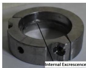
Figure 6. The fixture for clamping the horn
