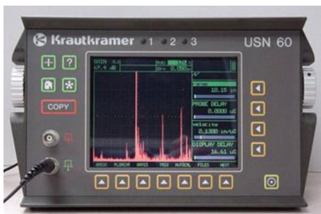
Figure 4: Ultrasonic device for tracking discontinuity
