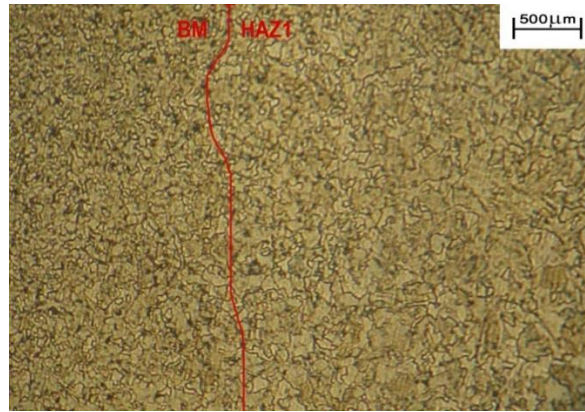
Figure 3. The microstructures variation from BM to HAZ
