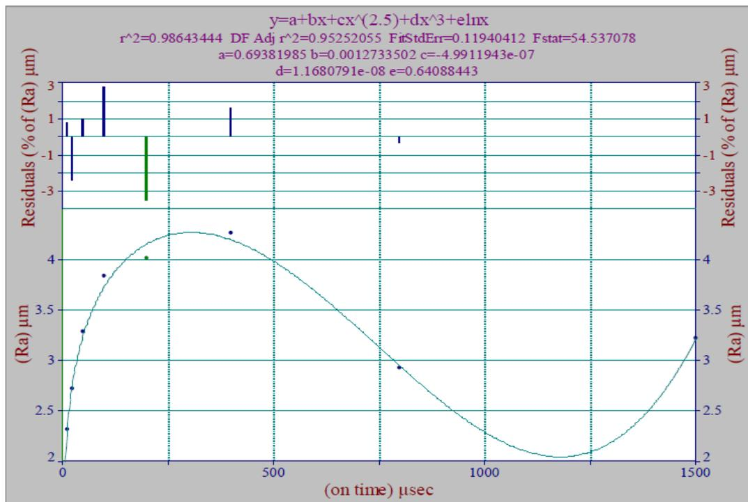
Figure5. Variation of surface roughness with on-time parameter (including errors)
