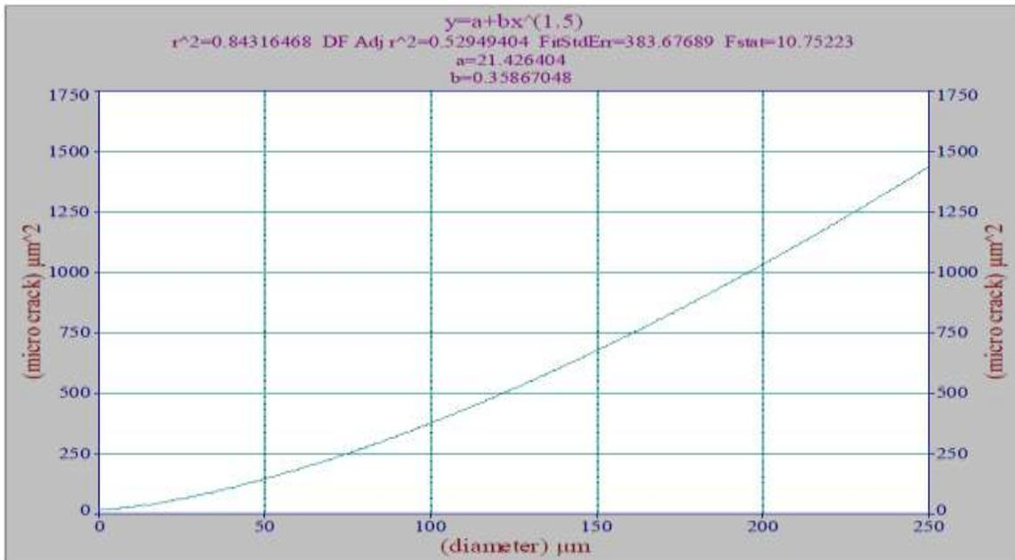
Figure10. Variation of the total surface of micro-cracks with the average grain diameter for varying off-time, voltage and current parameters
