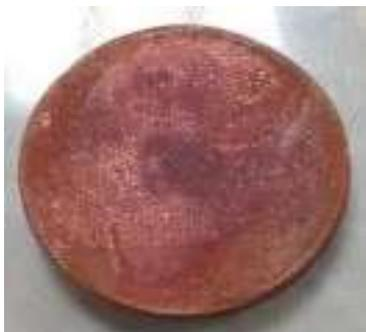
Figure4. Copper sample has been corroded after 20 hour
