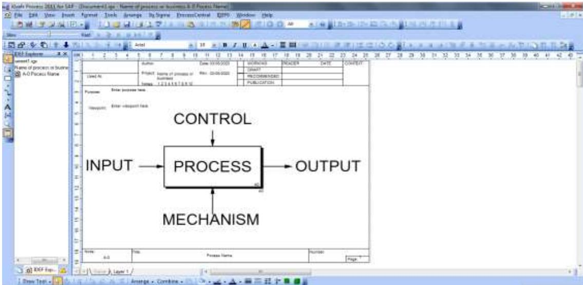
Figure1. IDEF0 process model Representation in iGRAF software
