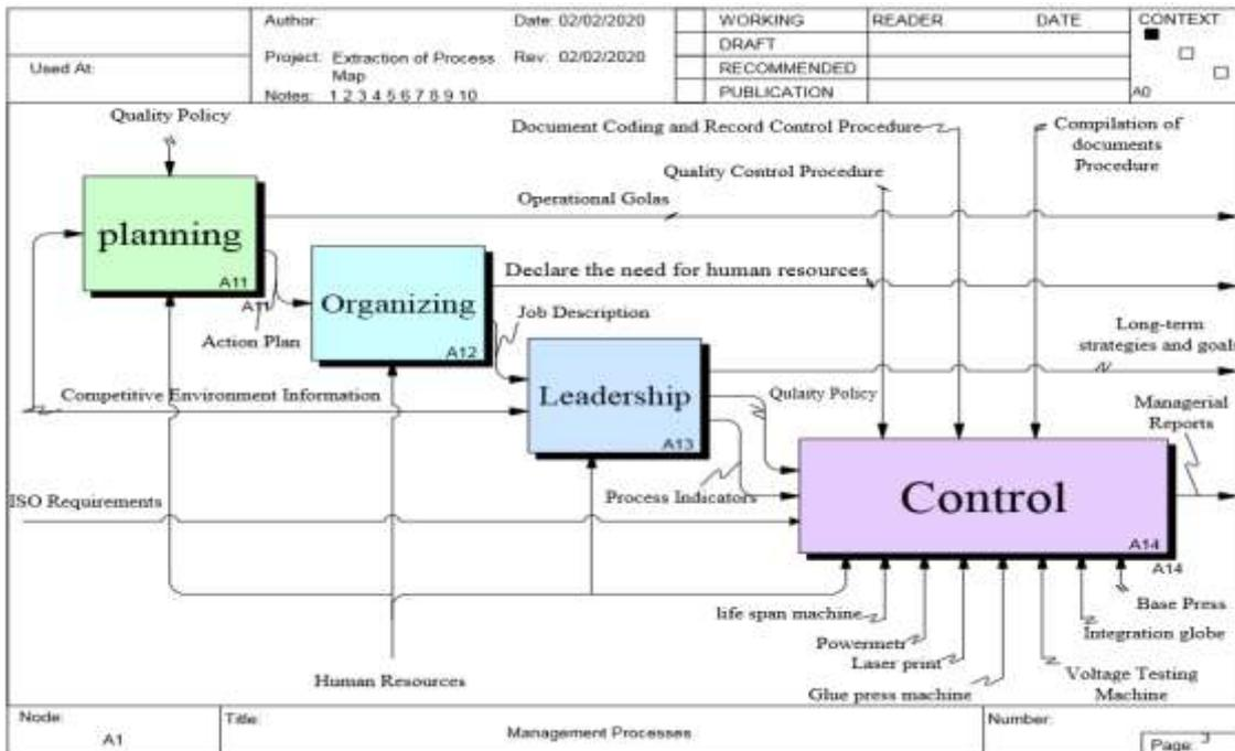
Figure5. Decomposition of box A1, Management Processes
