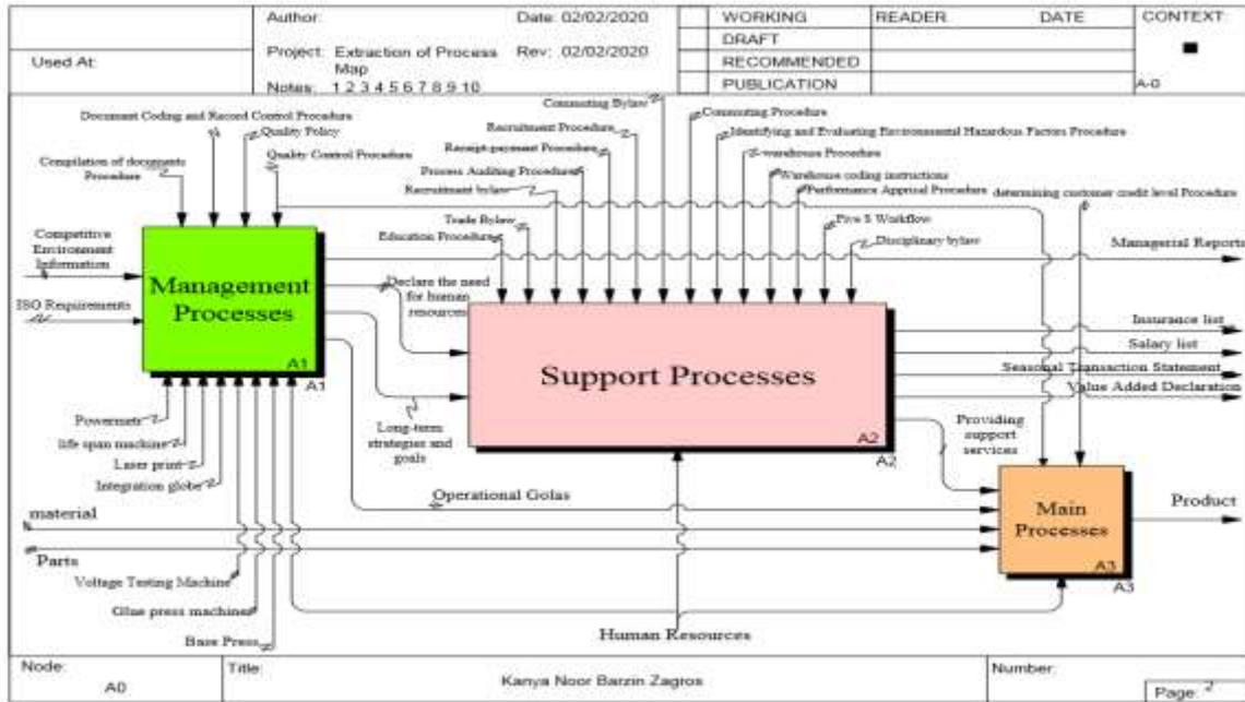
Figure4. Decomposition of box A0: Processes Map of KNBZ Company
