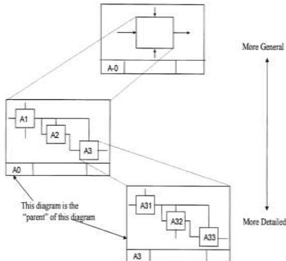
Figure 2. Decomposition construction of an IDEF0 model
