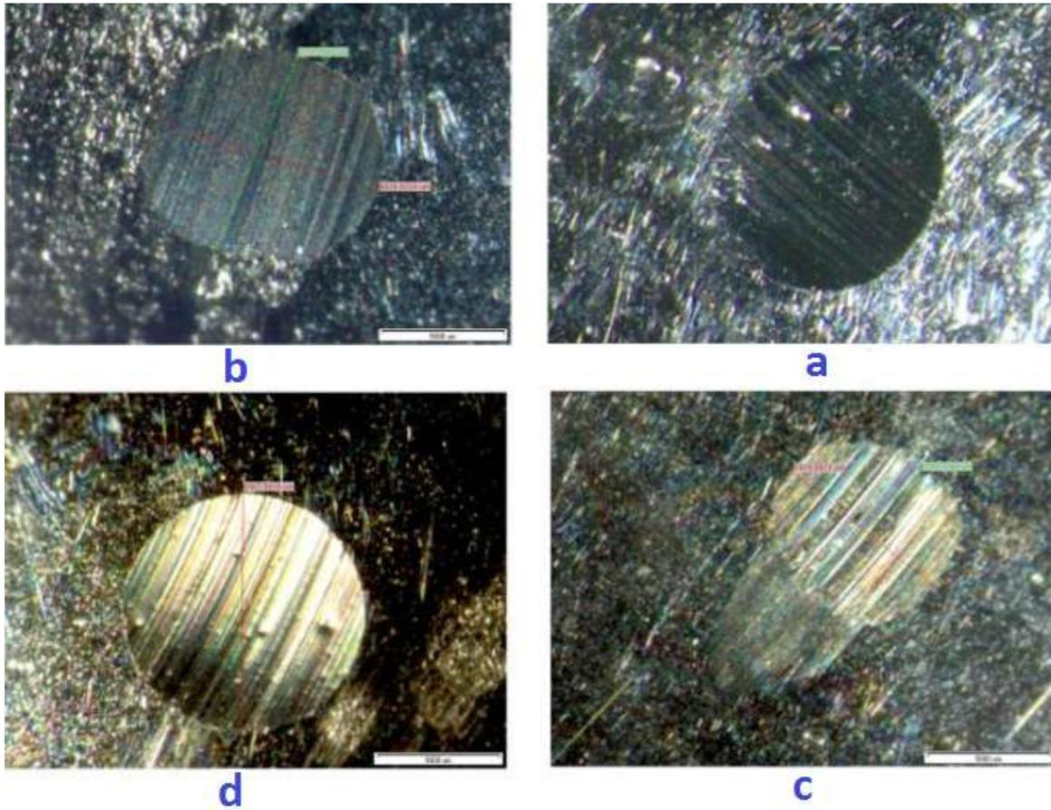
Figure10. The optical micrographs of worn surfaces for the B10 blend containing a) 0 ppm b) 25 ppm c) 50 ppm d) 75 ppm nanoparticles under 500 RPM
