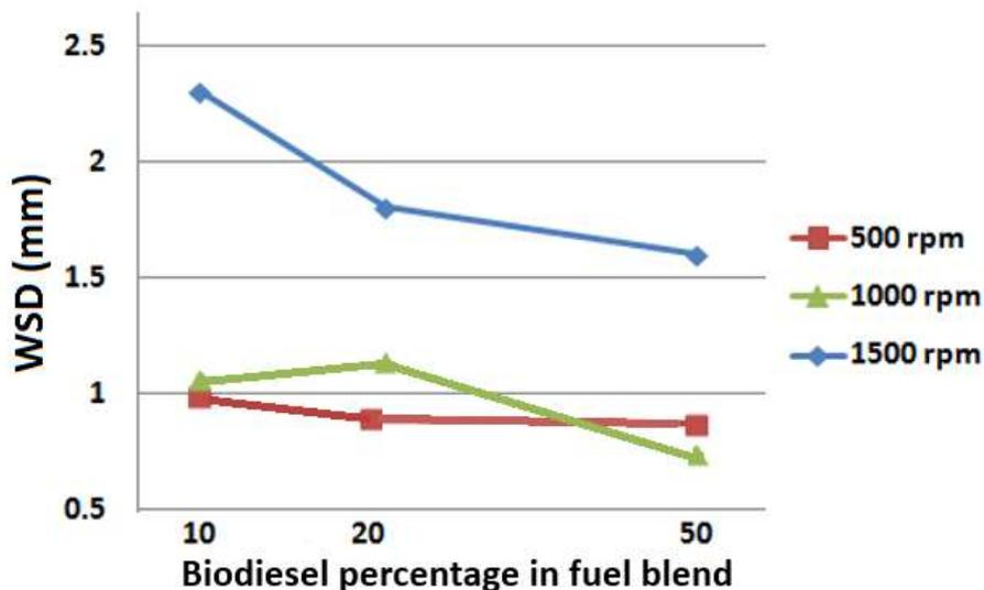
Figure9. Effect of biodiesel percentage in fuel blends containing 75 ppm nanoparticles on wear scar diameter
