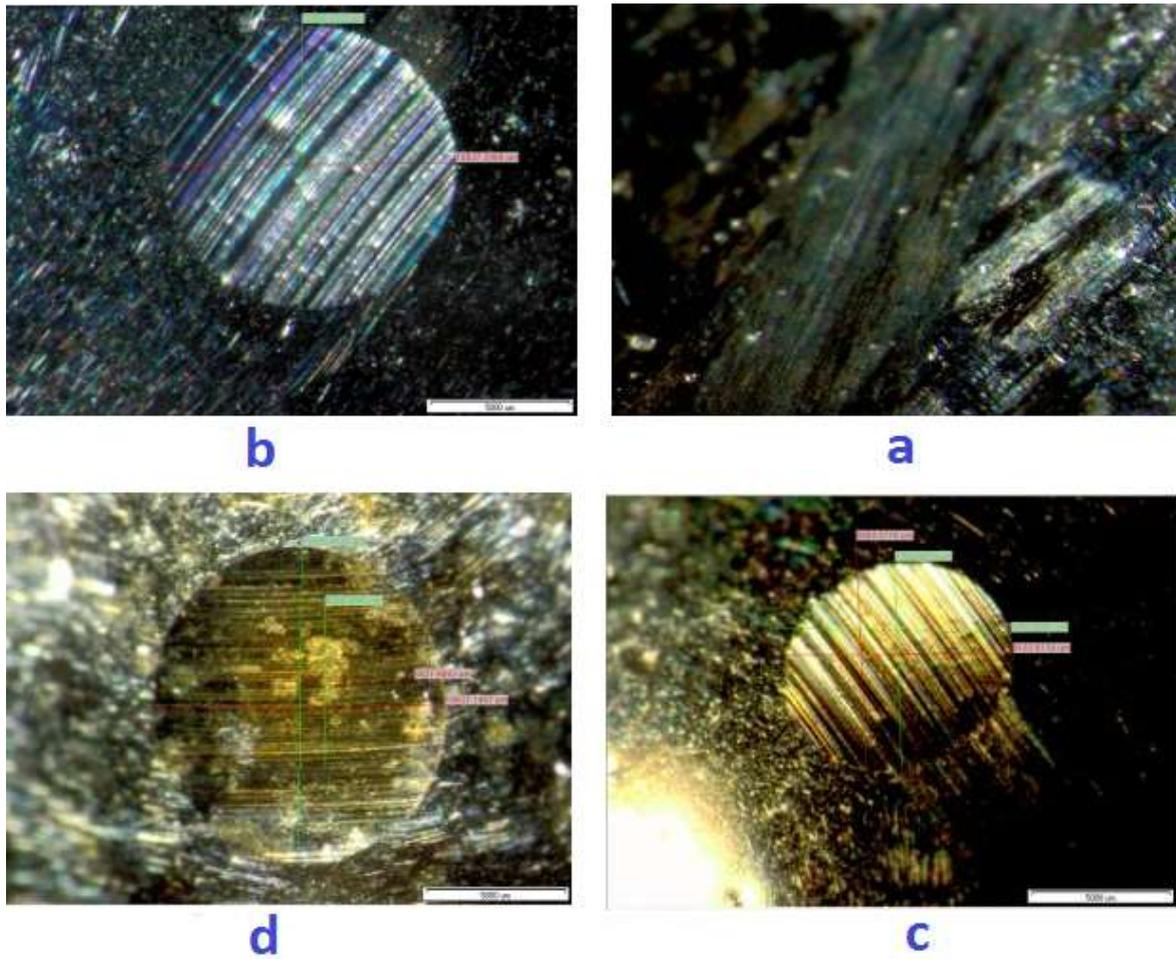
Figure13. The optical micrographs of worn surfaces for the B10 blend containing a) 0 ppm b) 25 ppm c) 50 ppm d) 75 ppm nanoparticles under 1000 RPM
