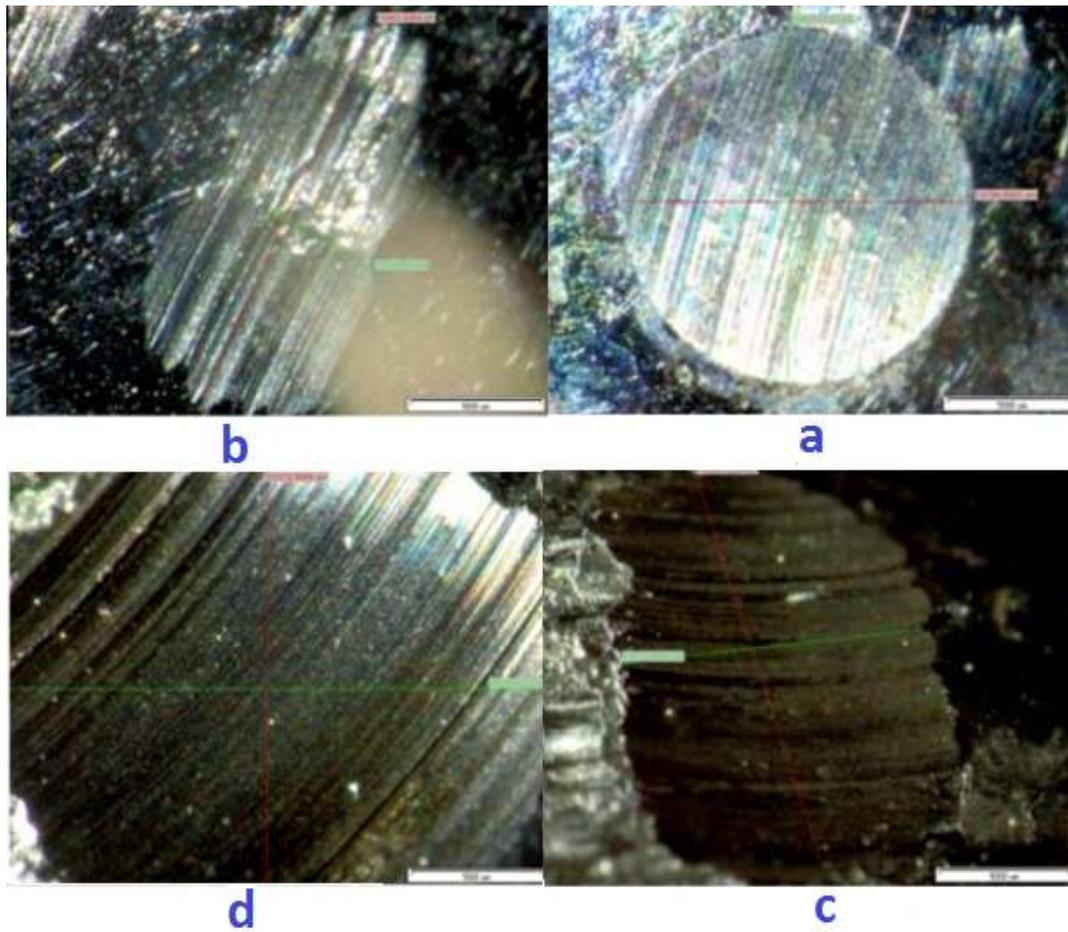
Figure17. The optical micrographs of worn surfaces for the B20 blend containing a) 0 ppm b) 25 ppm c) 50 ppm d) 75 ppm nanoparticles under 1500 RPM
