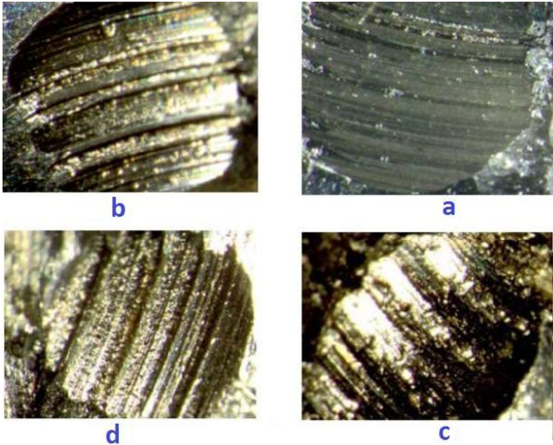
Figure16. The optical micrographs of worn surfaces for the B10 blend containing a) 0 ppm b) 25 ppm c) 50 ppm d) 75 ppm nanoparticles under 1500 RPM
