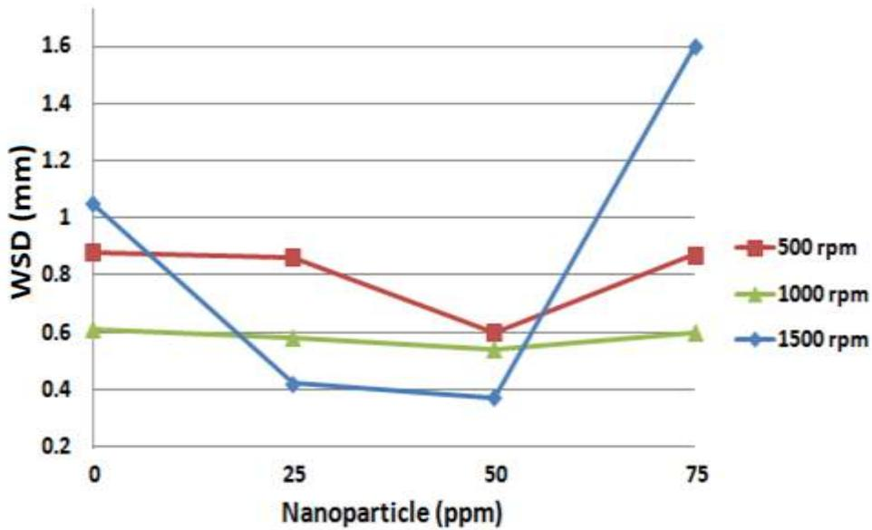
Figure5: The wear scar diameter versus different nanoparticles concentration in B50 blend
