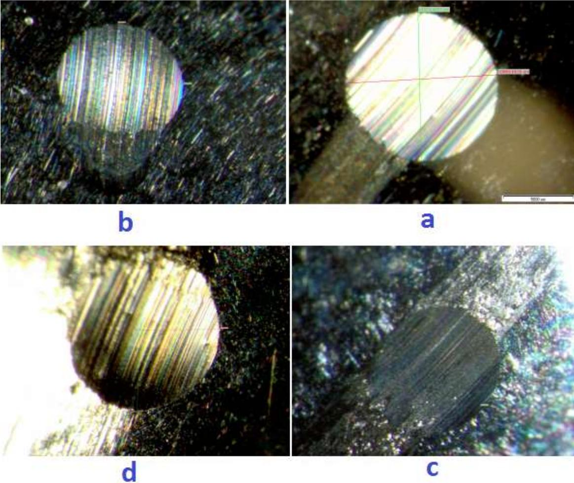
Figure14. The optical micrographs of worn surfaces for the B20 blend containing a) 0 ppm b) 25 ppm c) 50 ppm d) 75 ppm nanoparticles under 1000 RPM
