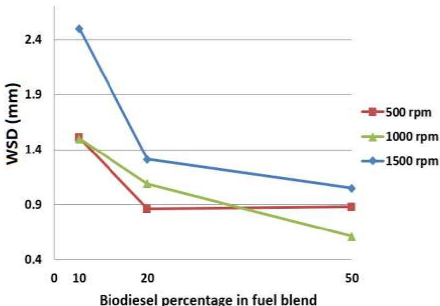
Figure6. Effect of biodiesel percentage in fuel blends without nanoparticles on wear scar diameter
