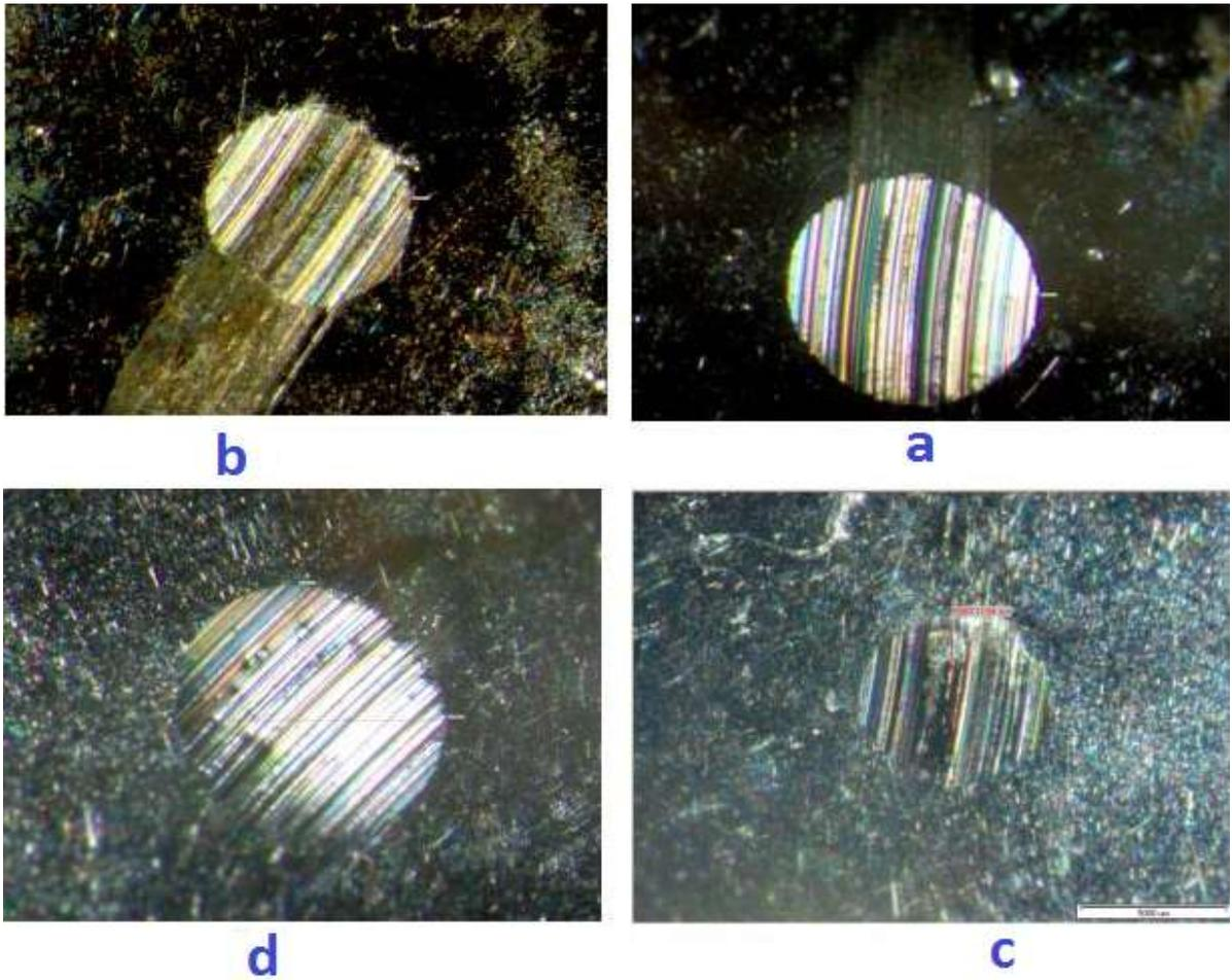
Figure15. The optical micrographs of worn surfaces for the B50 blend containing a) 0 ppm b) 25 ppm c) 50 ppm d) 75 ppm nanoparticles under 1000 RPM
