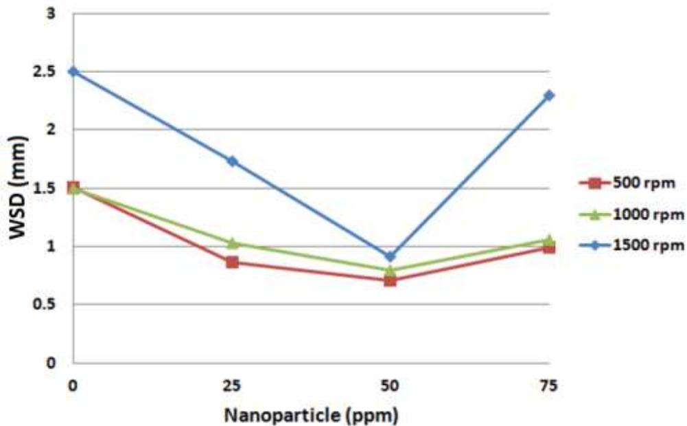
Figure3. The wear scar diameter versus different nanoparticles concentration in B10 blend
