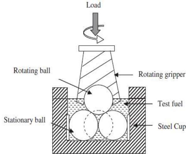
Figure2. A schematic diagram of the 4-ball wear tribo-tester [22]
