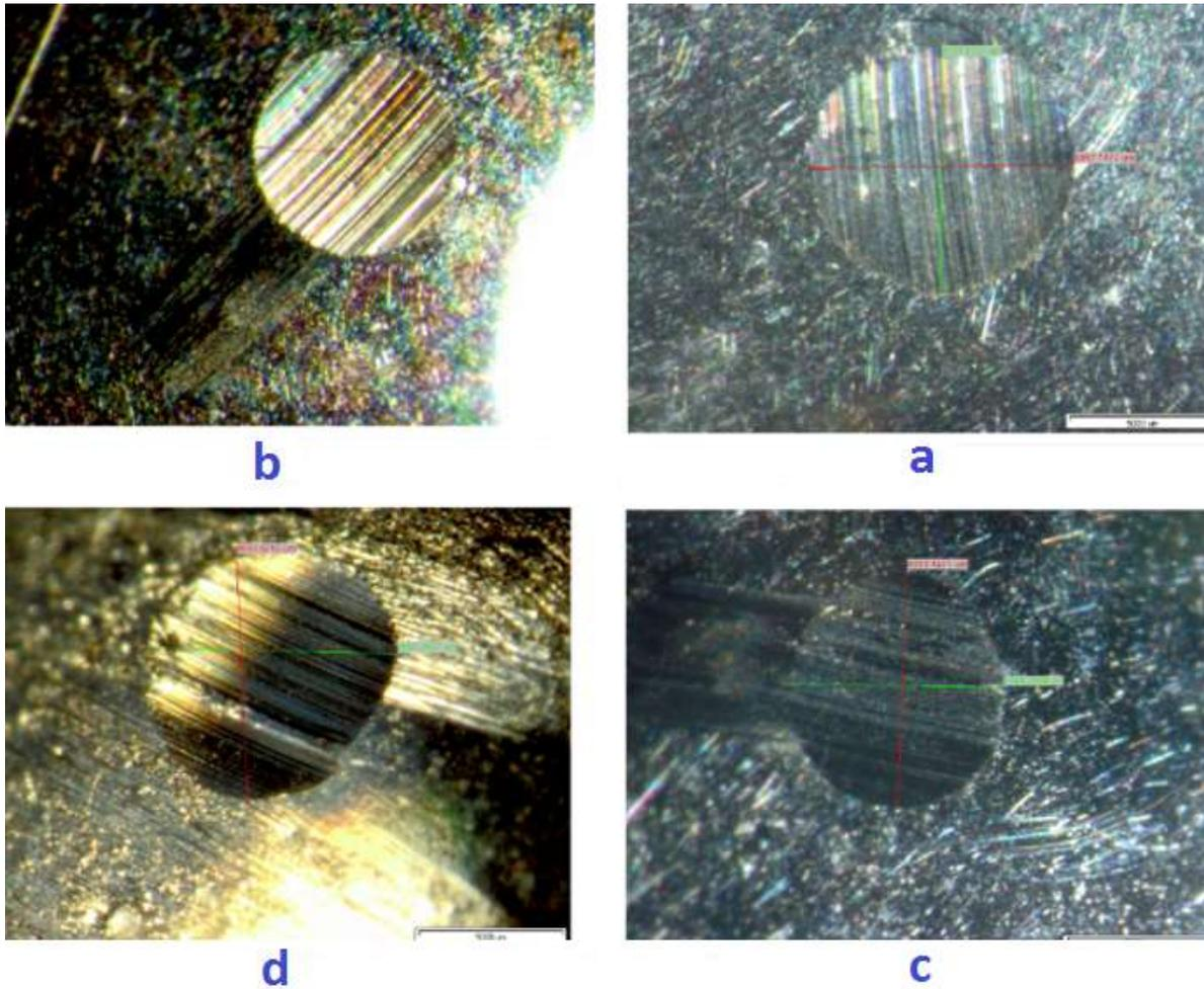
Figure11. The optical micrographs of worn surfaces for the B20 blend containing a) 0 ppm b) 25 ppm c) 50 ppm d) 75 ppm nanoparticles under 500 RPM
