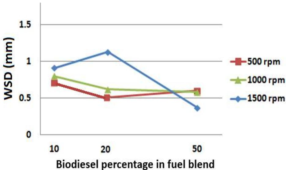
Figure8. Effect of biodiesel percentage in fuel blends containing 50 ppm nanoparticles on wear scar diameter
