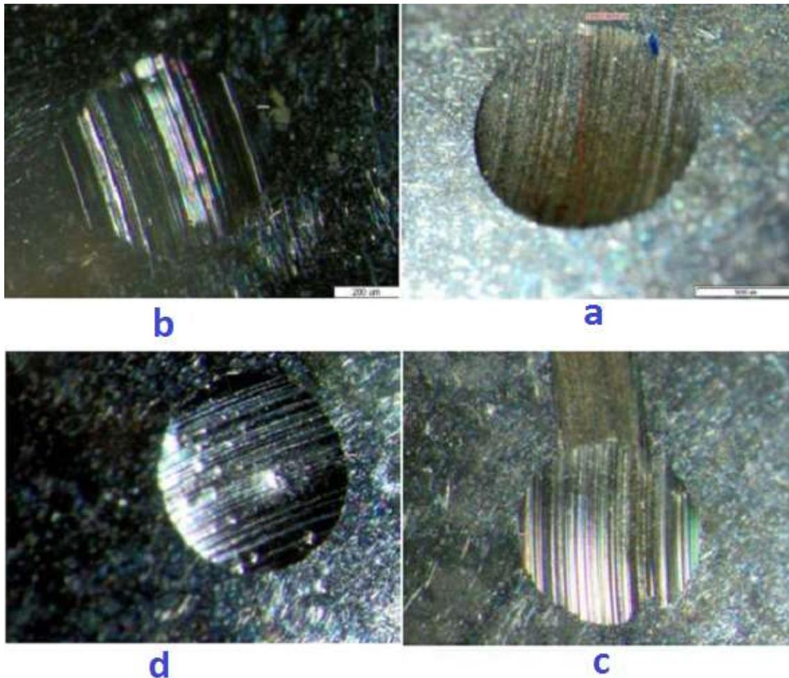
Figure18. The optical micrographs of worn surfaces for the B50 blend containing a) 0 ppm b) 25 ppm c) 50 ppm d) 75 ppm nanoparticles under 1500 RPM
