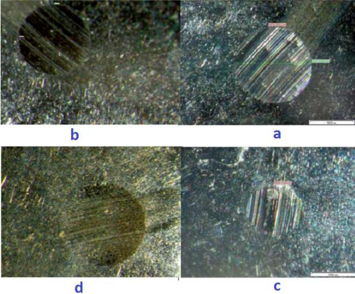
Figure12. The optical micrographs of worn surfaces for the B50 blend containing a) 0 ppm b) 25 ppm c) 50 ppm d) 75 ppm nanoparticles under 500 RPM
