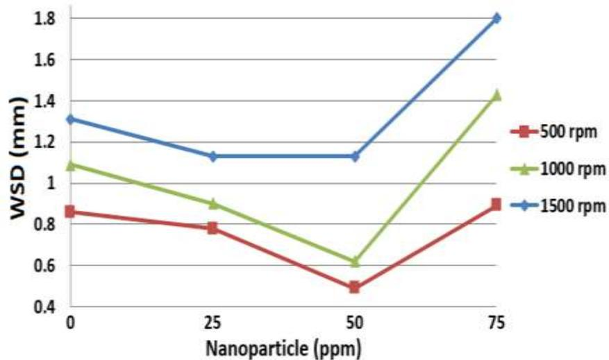
Figure4. The wear scar diameter versus different nanoparticles concentration in B20 blend
