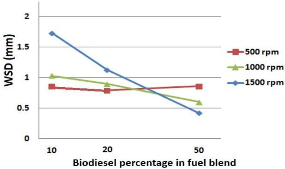
Figure7. Effect of biodiesel percentage in fuel blends containing 25 ppm nanoparticles on wear scar diameter
