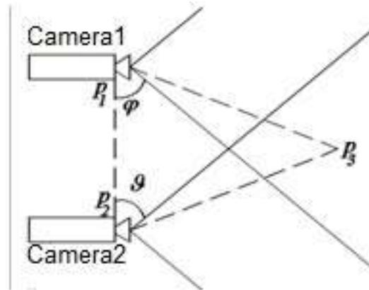
Figure5. Camera Positions in inactive stereo vision using two cameras
