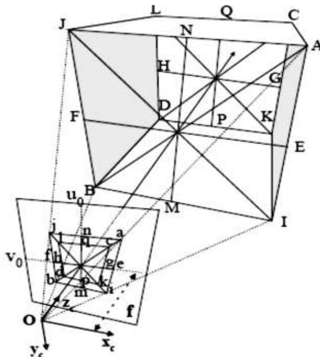
Figure 4. Using a specific box for calibration of the camera
