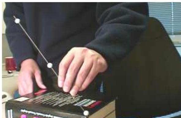
Figure3. Calibration of camera position using a set of the aligned points [3]
