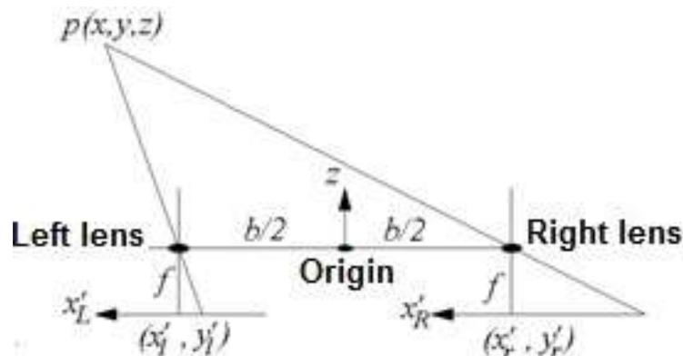
Figure6. Position of cameras and the measured point in coordinating axis located between the lens centers
