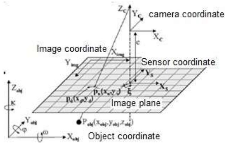
Figure1. Camera and object and coordinates [1]
