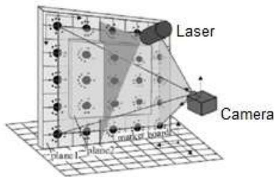
Figure2. Calibration of the camera position
