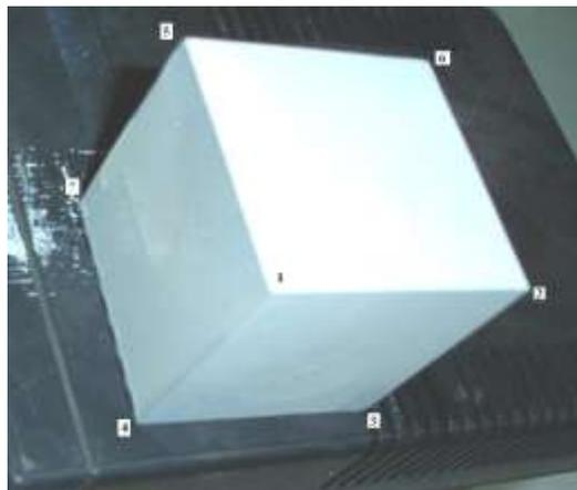
Figure7. The used object for calibration point specification
