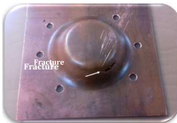
Figure4. A view of rupture after drawing
