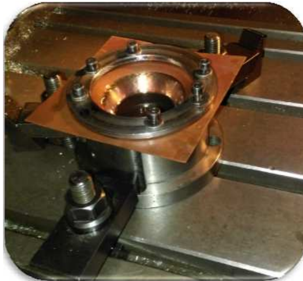
Figure2. A view of the sheet closure in the fixture and deformation of the sheet
