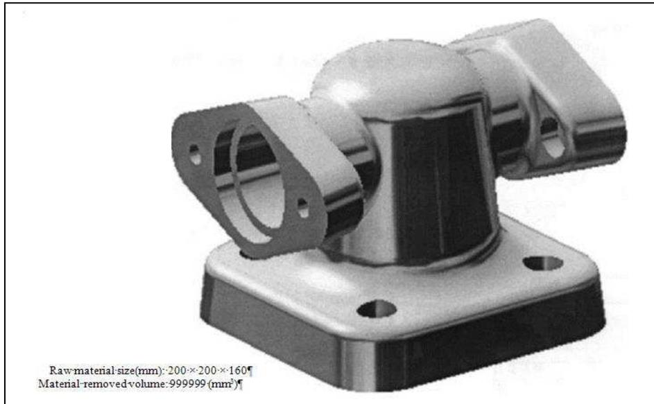
Figure6. Geometrical solid model of the part (Adopted from [19])
