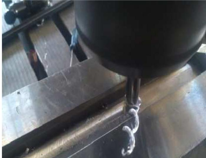
Figure3. Implementation of frictional stir welding process
