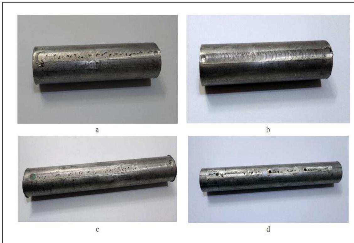
Figure4. Welded piece using frictional stir welding tube process: a) Rotational speed of 2000 rpm and welding speed of 12mm/min b) Rotational speed of 2500 rpm and welding speed of 8 mm/min c) Rotational speed of 2000 rpm and welding speed of 4 mm/min d) Rotational speed of 1600 rpm and welding speed of 8 mm/min
