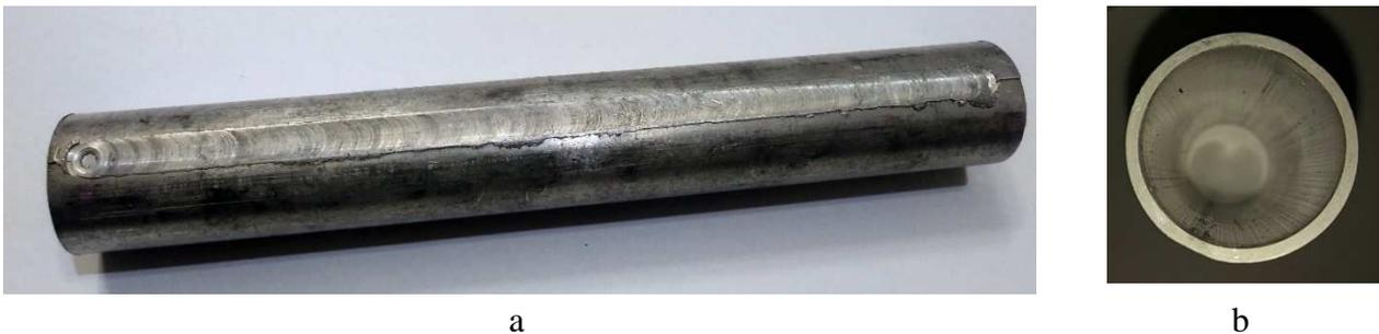
Figure6. Manufactured part in appropriate friction stir welding condition, rotation speed of 2500 rpm and welding speed of 4 mm/min a) The sound cylindrical part, b) cross section of the welded tube
