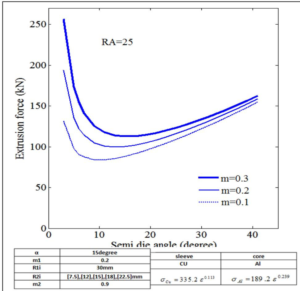
Figure6. effect of die angle in the extrusion force in various friction coefficients between the work piece and the die
