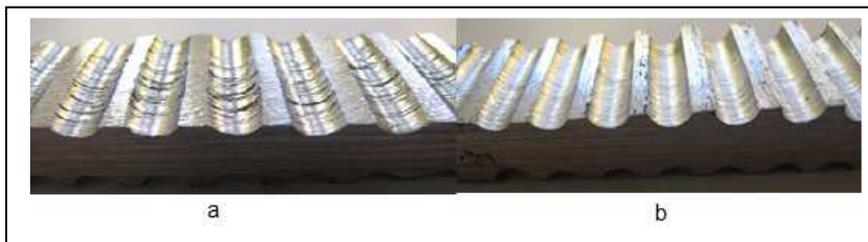
Figure12. The cross section of the workpiece a) in conventional drilling and b) in vibration assisted drilling
