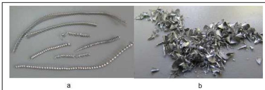
Figure13. The chips in a) conventional drilling and b) vibration assisted drilling
