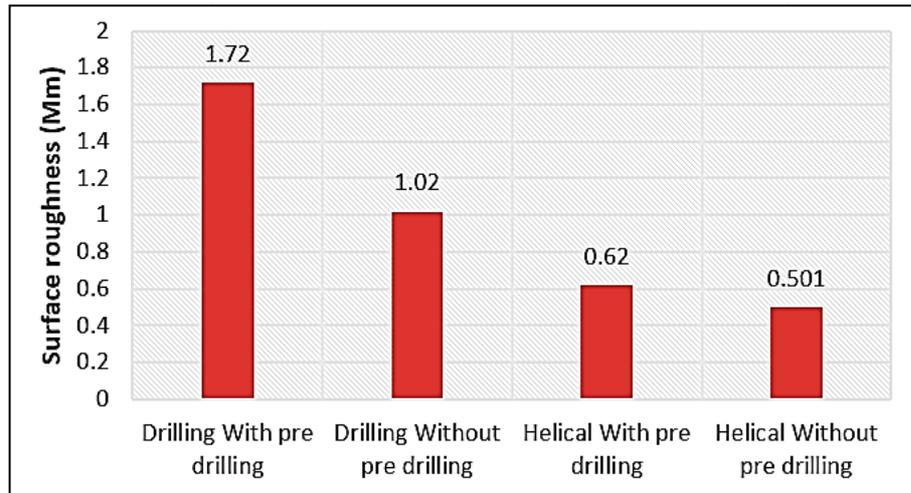
Figure6. The variations of surface roughness
