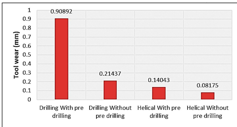
Figure5. Tool wear of different machining conditions
