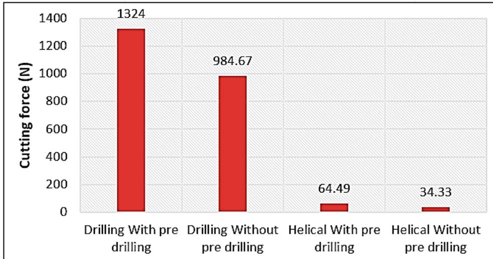
Figure7. The variation of cutting force in various processes
