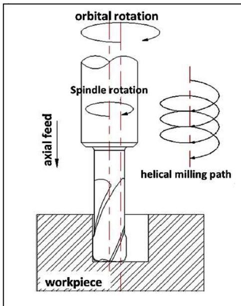
Figure2. Schematic of helical milling process [20]
