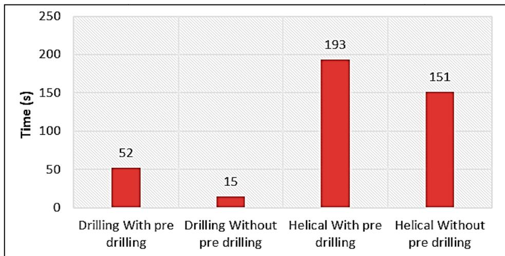
Figure8. The variation of machining time
