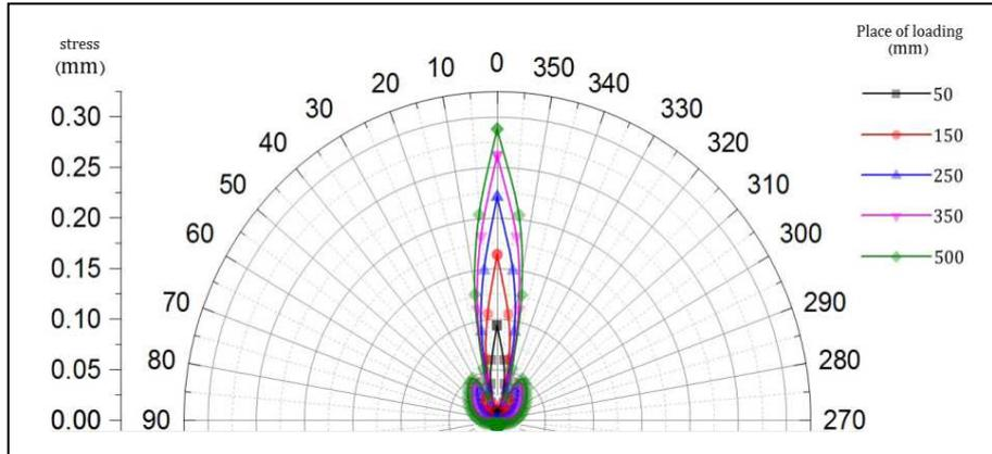
Figure9. Permanent displacement at circumferential direction of tube - thickness of 4 mm
