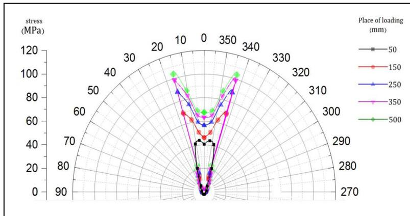
Figure7. residual stress changes in the circumferential of tube - thickness of 6.3 mm
