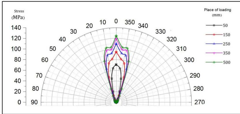
Figure5. residual stress changes in the circumferential of tube - thickness of 4 mm
