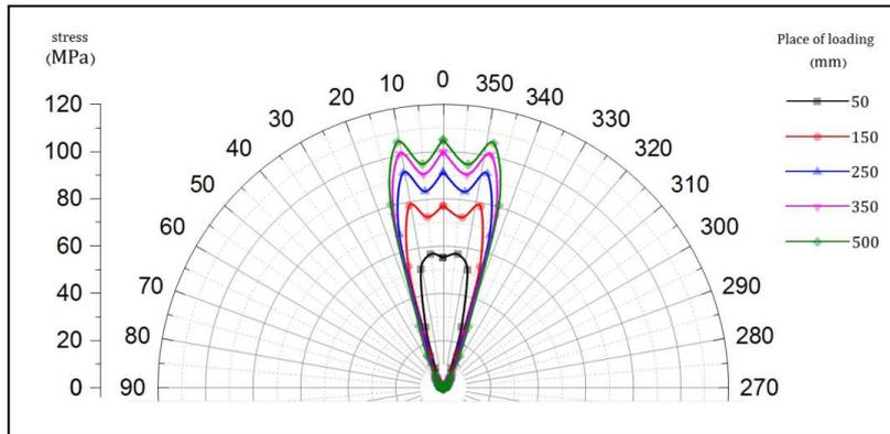
Figure6. residual stress changes in the circumferential of tube - thickness of 5 mm
