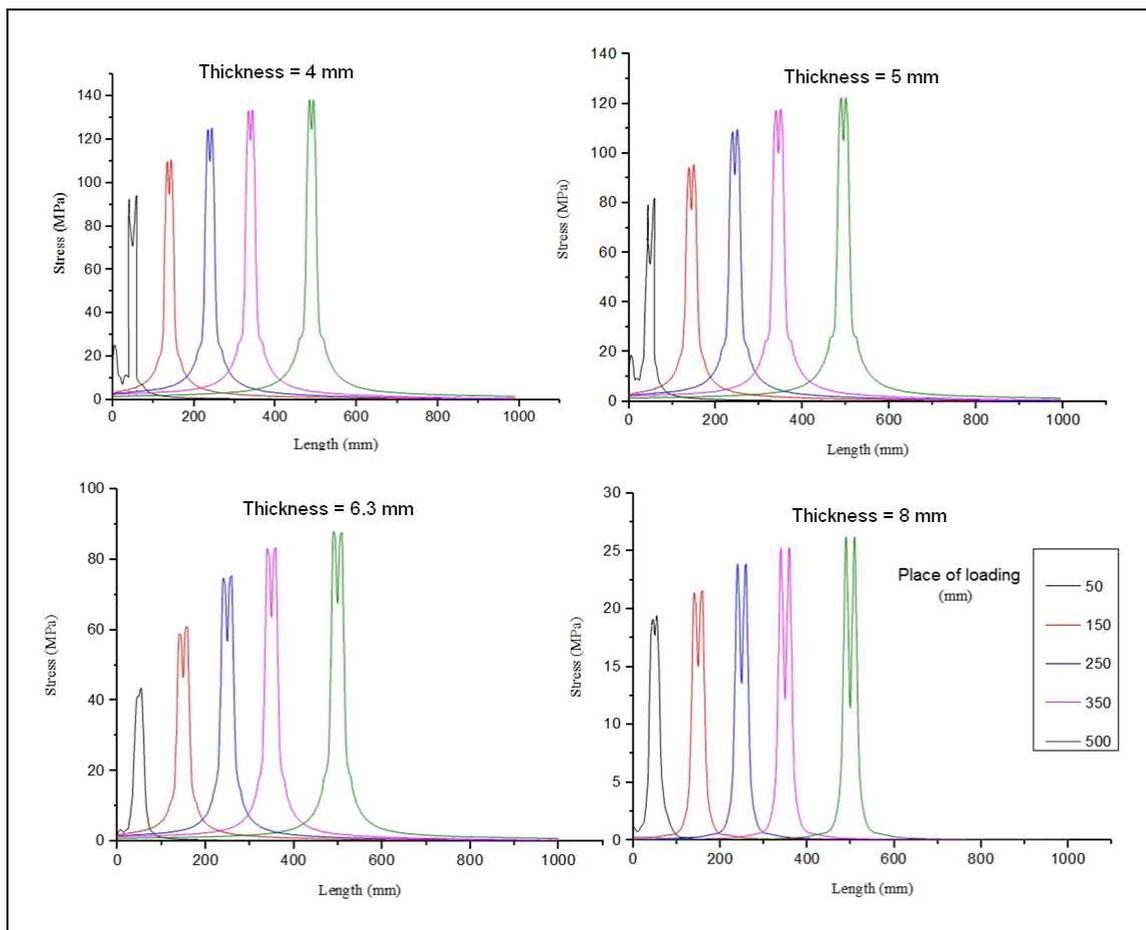
Figure3. changes in residual stress in tubes with diferent thickness
