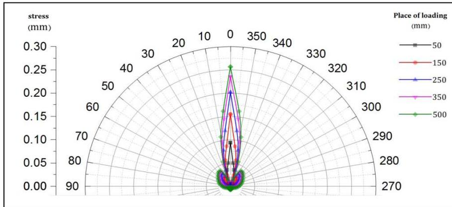
Figure 10. Permanent displacement at circumferential direction of tube - thickness of 5 mm
