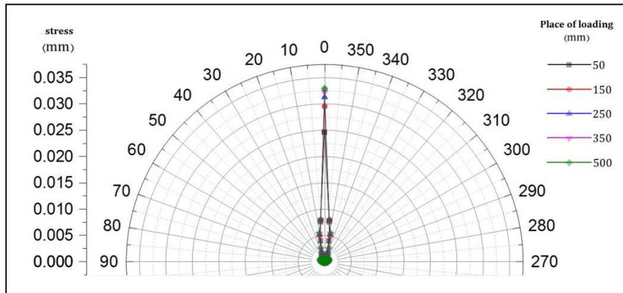
Figure 12. Permanent displacement at circumferential direction of tube - thickness of 8 mm
