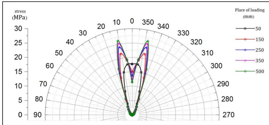
Figure8. residual stress changes in the circumferential of tube - thickness of 8 mm
