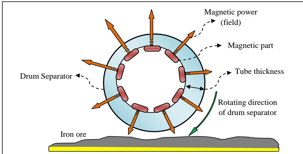
Figure1. The effect of magnetic gap on separation the iron from iron ore
