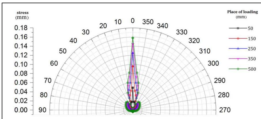
Figure 11. Permanent displacement at circumferential direction of tube - thickness of 6.3 mm
