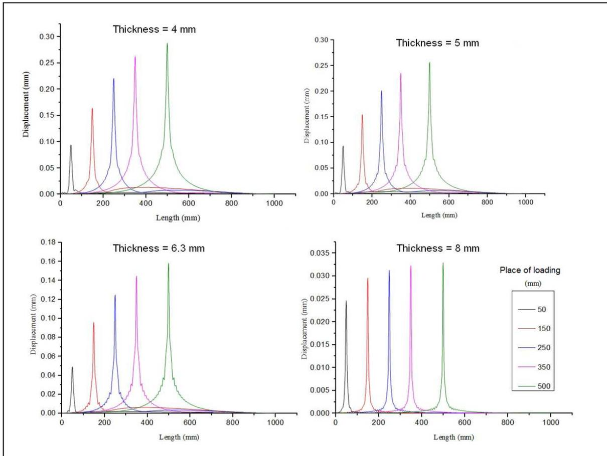
Figure4. changes in permanent displacement in tubes with diferent thickness
