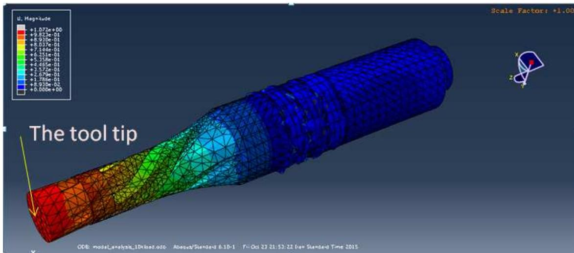
Figure2. Mode shape at 22363 Hz
