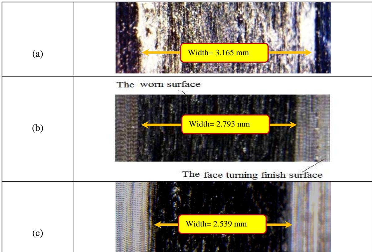
Figure 6. Morphologies of wear scars of three kinds of un-textured surface and textured surfaces according to the condition of  $V_c = 35$  m/min,  $f = 0.205$  mm/rev and UAT<sub>d1</sub>, after the distance of 300 m at the velocity of 0.2 m/s; (a) CT, (b) UAT<sub>a1</sub>, (c) UAT<sub>a2</sub>.
