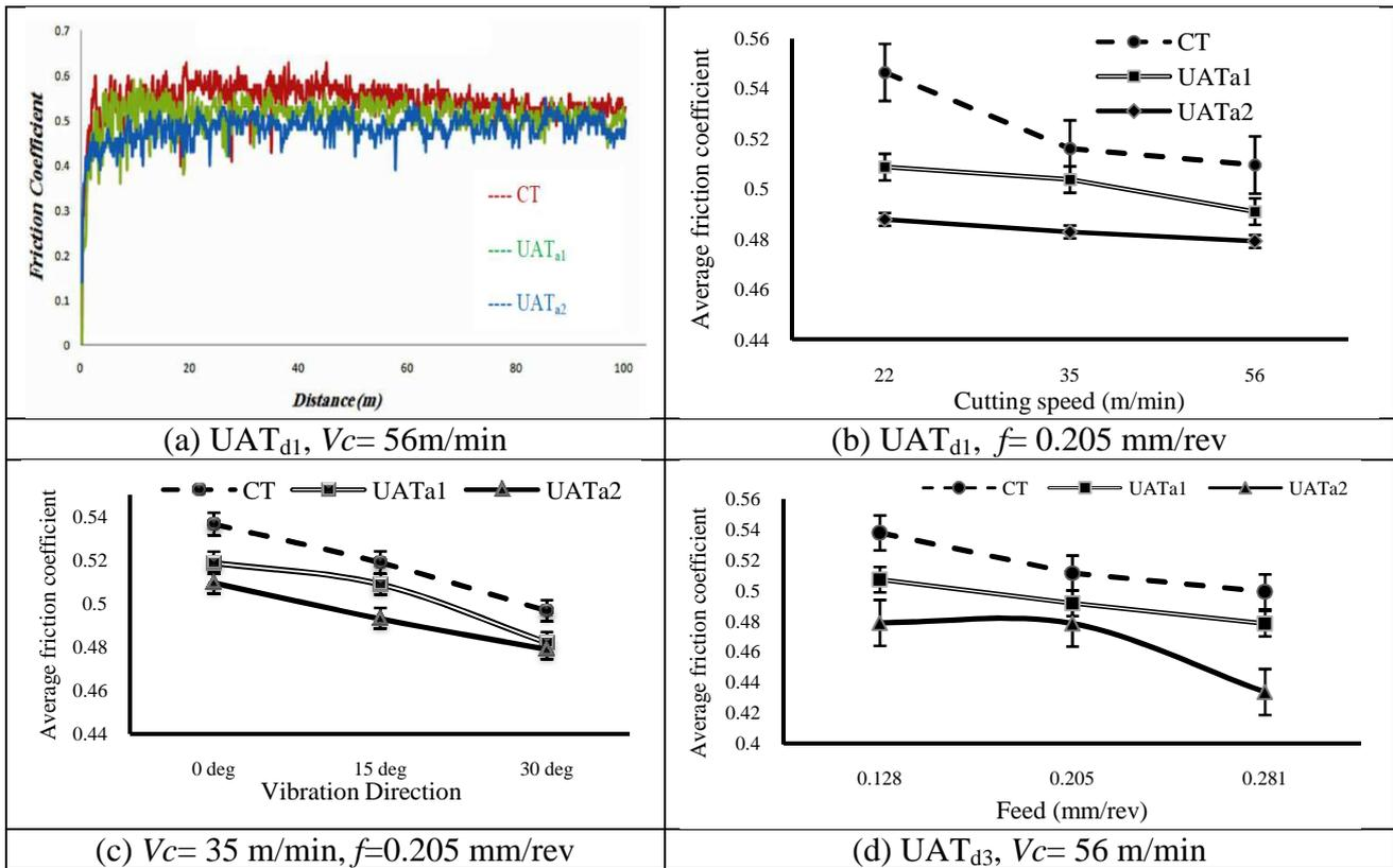
Figure 5. a) Measurement of the friction coefficient, comparison of friction coefficient in CT, UAT<sub>a1</sub> and UAT<sub>a2</sub> with the different values of (b) cutting speed, (c) vibration direction, (d) feed.
