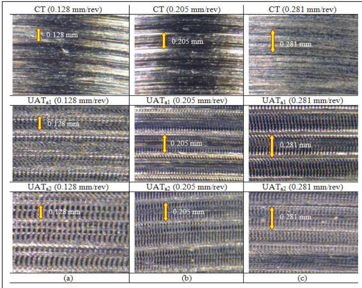
Figure3. Comparison of surface texture for the vibration angle of  $15^\circ$  according to the influence of  $V_c$  of 56 m/min and different feed levels.
