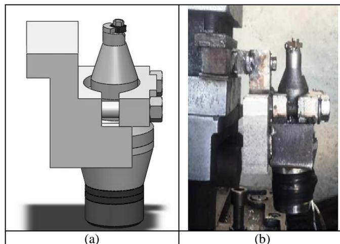
Figure 1. a) 3D model of the designed vibro-tool sets, installation modes of the fixture.
