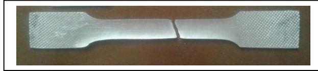
Figure5.The sample of tensile test
