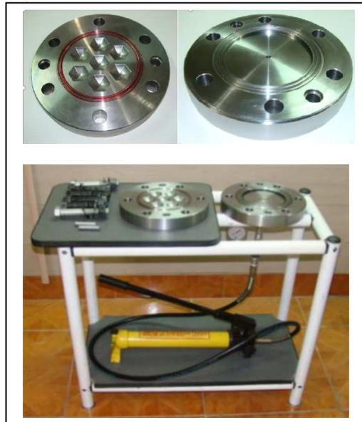
Figure7. The mold and sets machine hydroforming [4]
