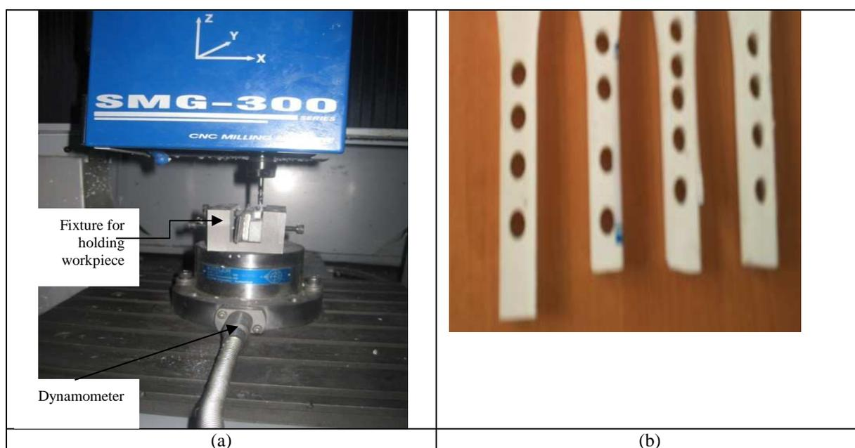
Figure1. a)Actual machining operation, b)Drilled work-pieces
