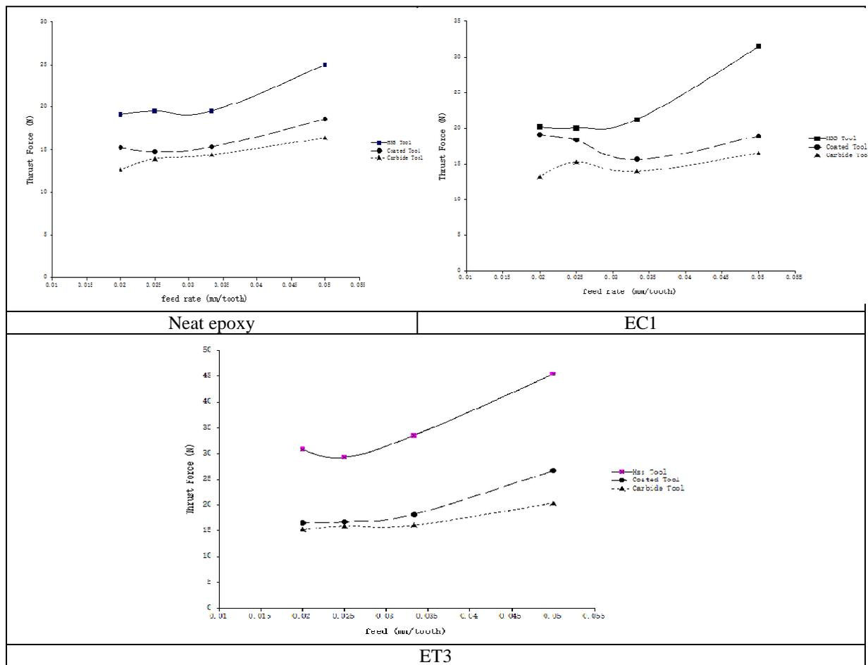
Figure3. Thrust force as function of feed rate and tool type for neat epoxy, EC1 and ET3 (Spindle speed=2000 rpm)
