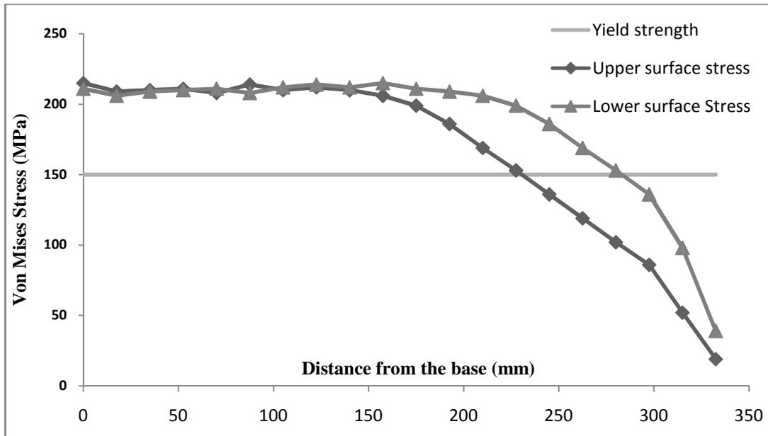
Figure. 14. Von Mises stress distribution on length
