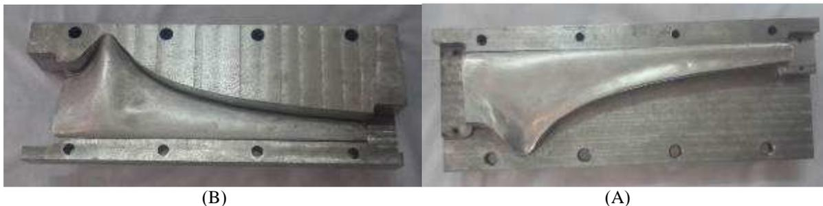
Figure 3. The blades fit within (A) the upper half mold (B) the lower half mold
