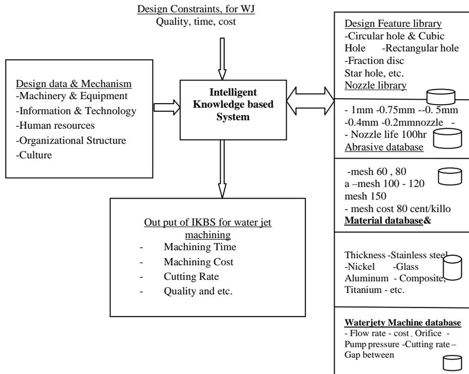
Figure6. Architecture of IKBS for water jet machining
