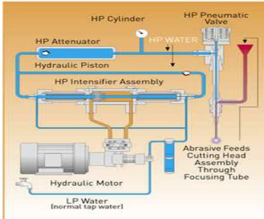
Figure 2. Components of a typical water jet machining
