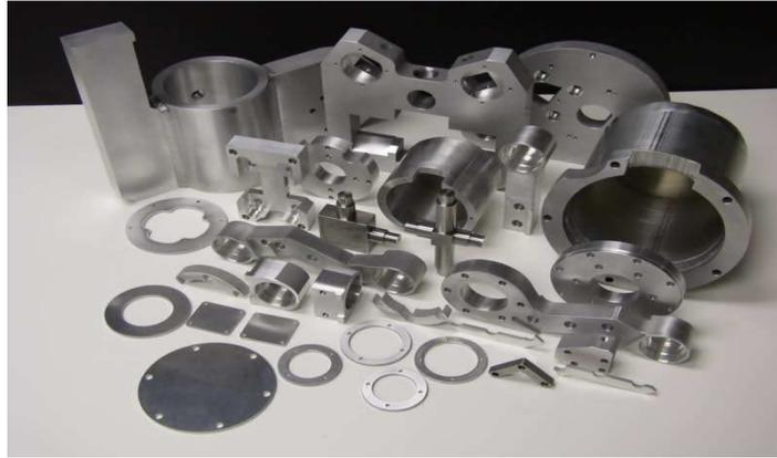
Figure5. Examples parts machined by water jet
