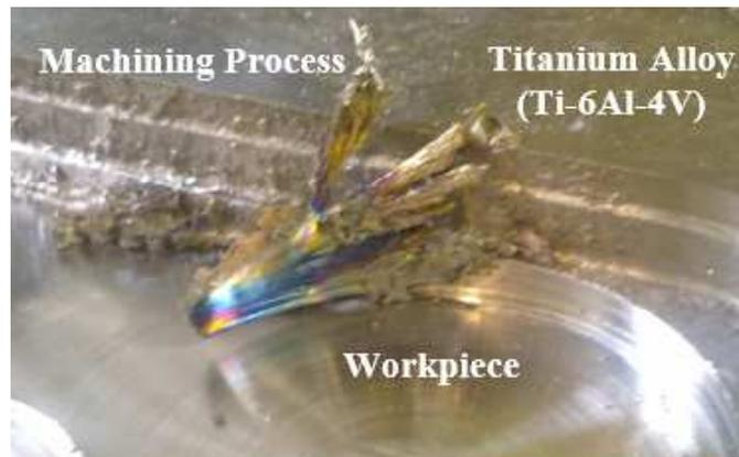
Figure1. Titanium alloy is work hardening material
