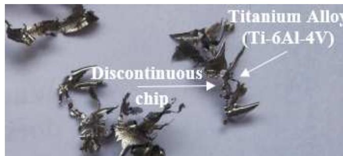
Figure5. Discontinuous chip formation during milling process
