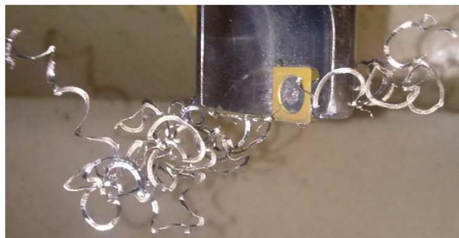
Figure3. High thermal between cutting tool and work-piece surface leads welding
