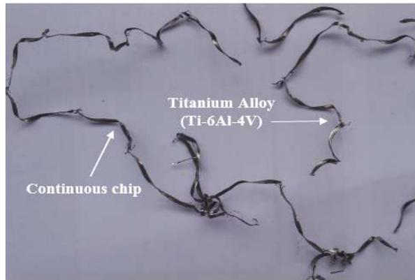
Figure4. Continuous chip formation during milling process
