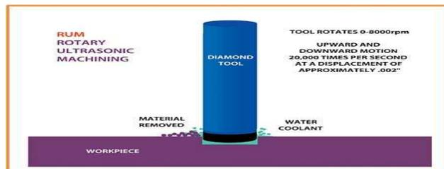
Figure4. Rotary ultrasonic machining process
