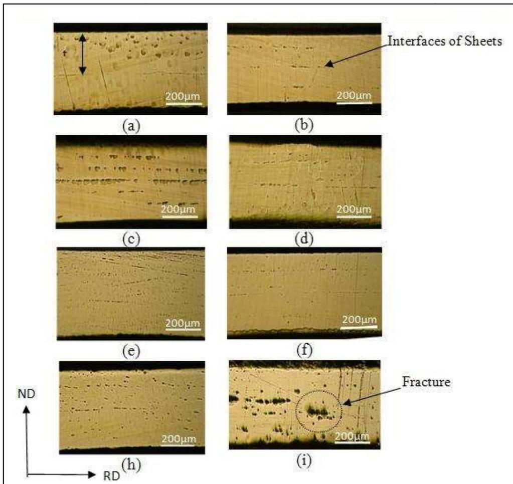
Figure3. Micrograph images of the ARB sheet viewed from TD and ND. (a) cycle 1, (b) cycle 2, (c) cycle 3, (d) cycle 4, (e) cycle 4, (f) cycle 5, (g) cycle 6, (h) cycle 7, (i) cycle 8
