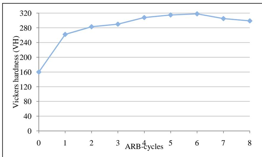
Figure10. Changes in Vickers hardness of the commercial purity Ti ARB-processed by various cycles
