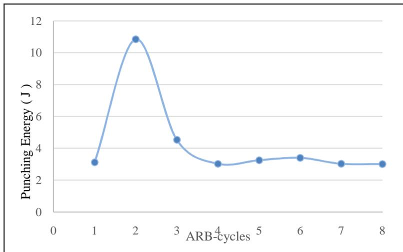
Figure9. Punching energy of different ARB cycles
