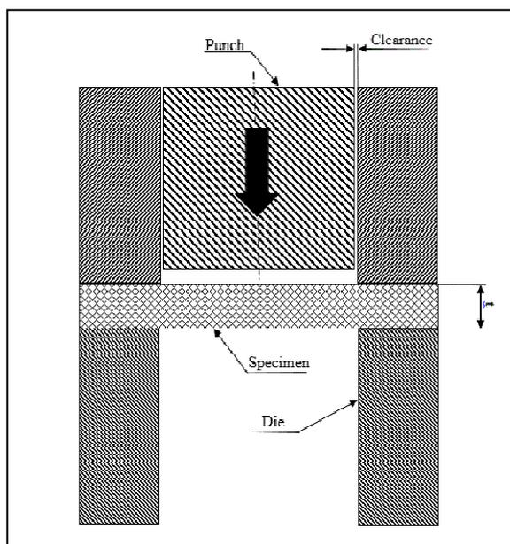
Figure4. Schematic conception of the punch test equipment
