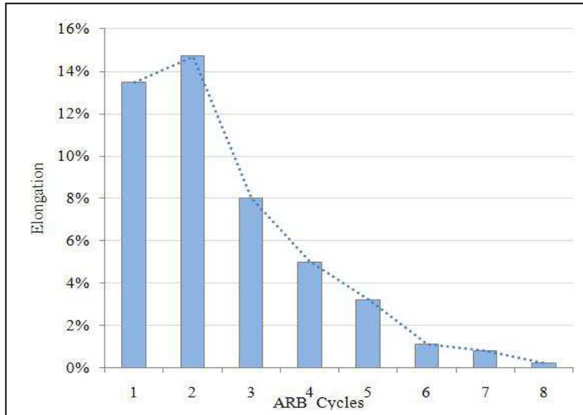
Figure8. Elongation of the commercial purity Ti ARB-processed by various cycles
