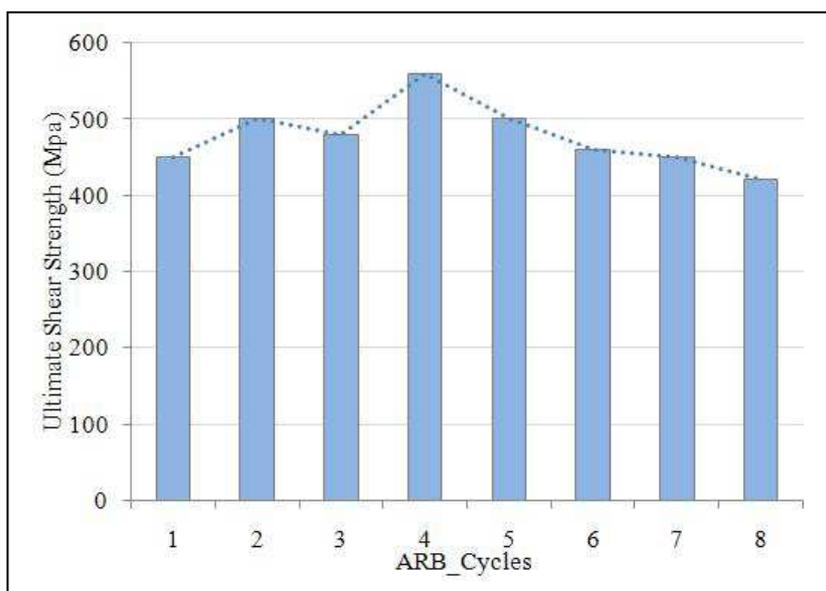
Figure7. Ultimate Shear Strength (USS) of the commercial purity Ti ARB-processed by various cycles
