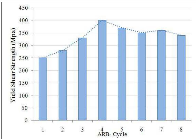
Figure6. Yield Shear Strength (YSS) of the commercial purity Ti ARB-processed by various cycles
