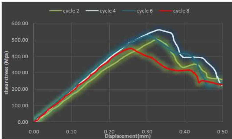
Figure5. Comparison of shear stress –displacement curve of different ARB cycles
