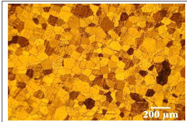
Figure2. Microstructures on longitudinal sections of the commercial purity Ti
