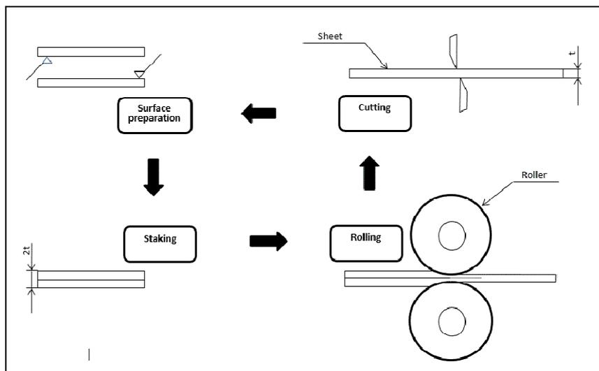
Figure1. Schematic illustration showing the principle of the accumulative roll-bonding process
