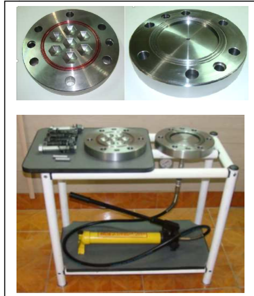
Figure7. The mold and sets machine hydroforming [4]
