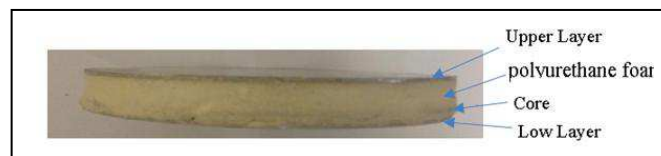
Figure10. Proposed honeycomb sandwich panels filled with polyurethane foam
