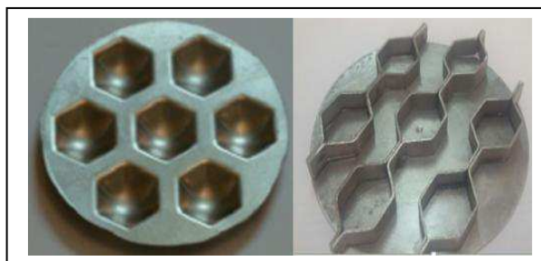
Figure4. (a)The proposed middle core formed by hydroforming process,(b) Traditional sample [4]
