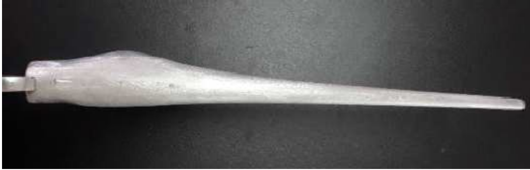
Figure 4. final form of blade obtained by hydroforming process
