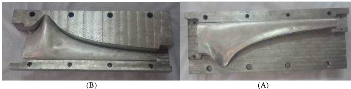
Figure 3. The blades fit within (A) the upper half mold (B) the lower half mold
