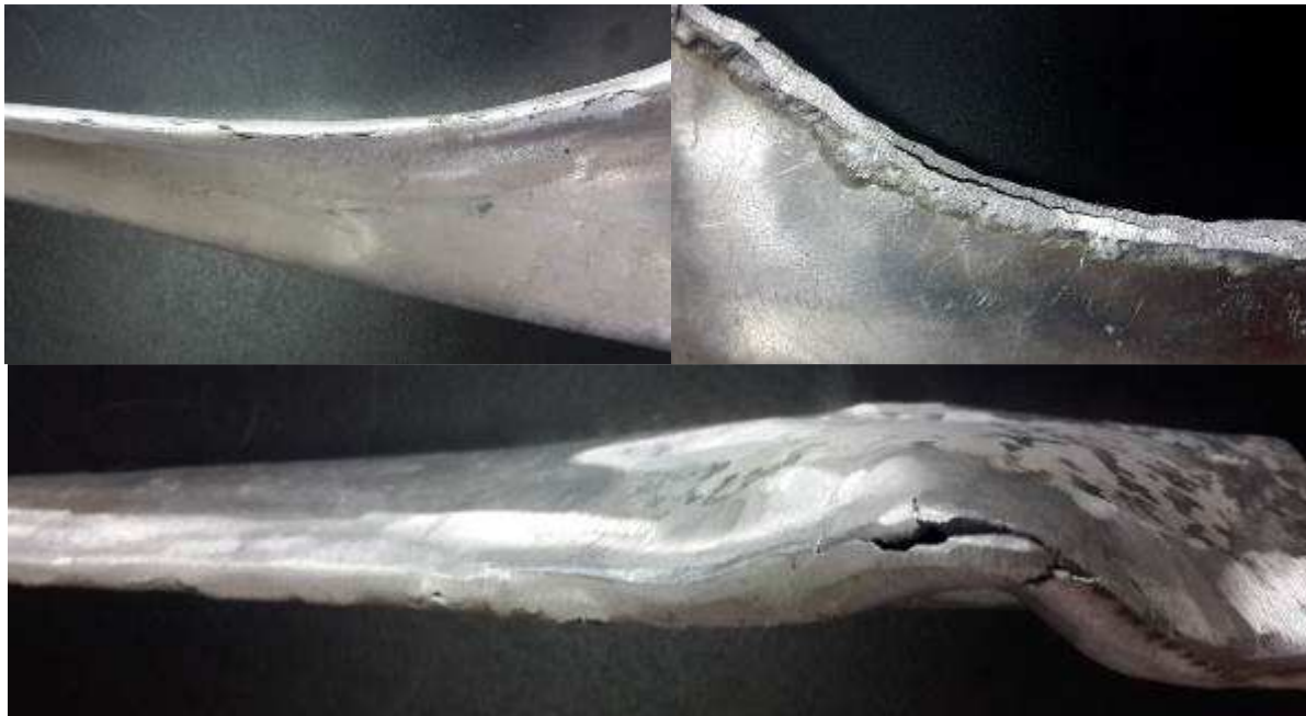
Figure 1. View of bursting piece of the Seam welding
