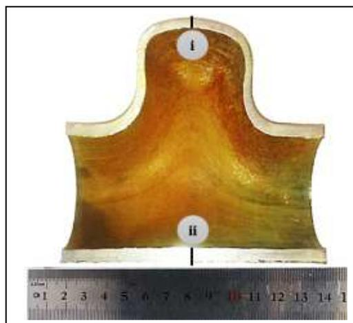
Figure14. Axial cross section of experimental T-branch sample
