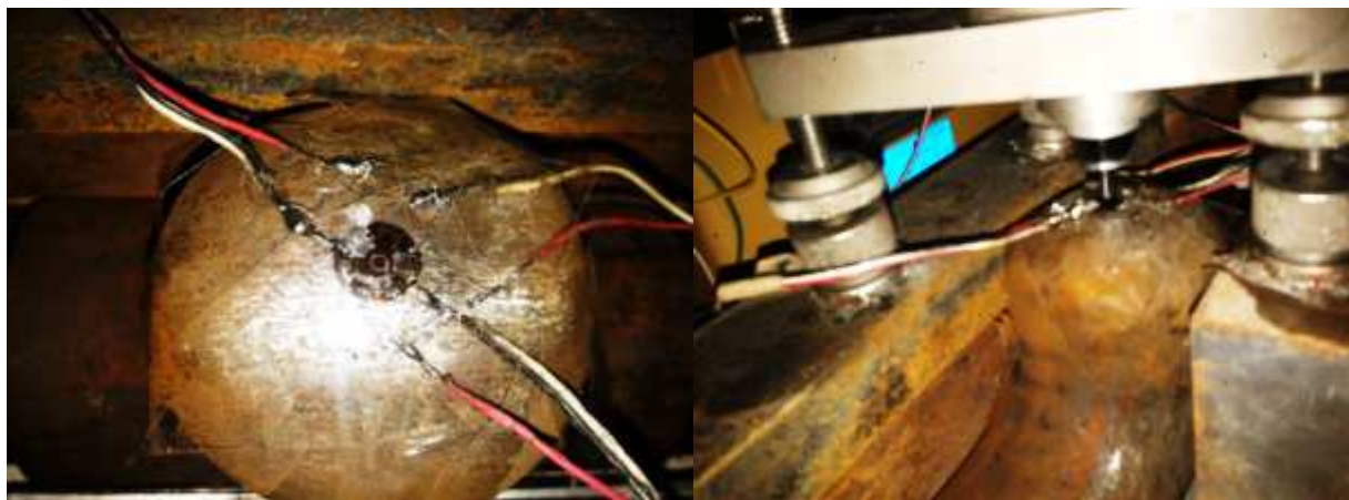
Figure3. Experimental Test of Residual Stress Measurement
