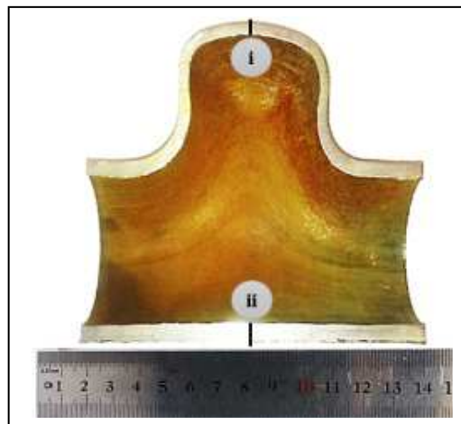
Figure14. Axial cross section of experimental T-branch sample
