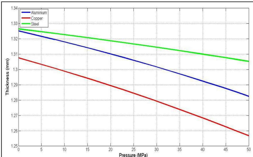
Figure15. The Effect of the Tube Material on the Tube Thickness
