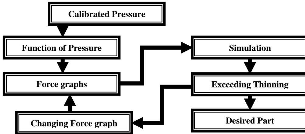
Figure9. The Control strategy applied to the Software
