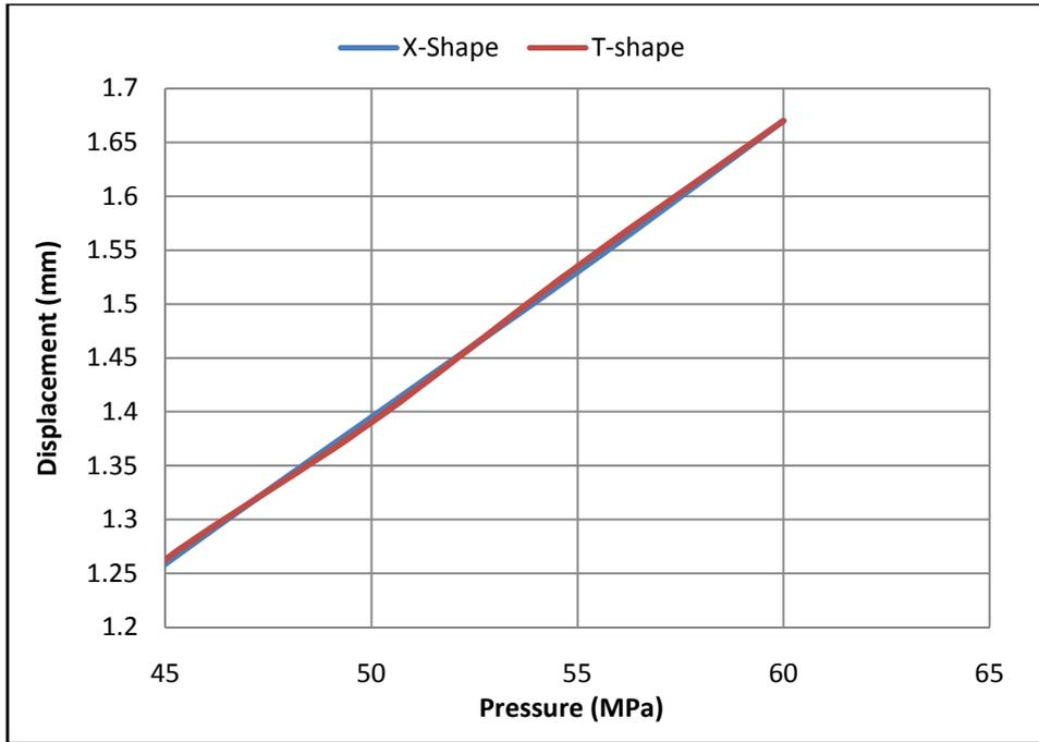
Figure7. Effect of the Pressure Changes Comparison in T-Shape and X-Shape in Hydroforming Process
