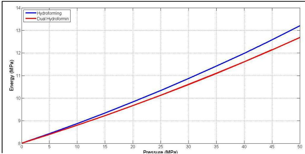
Figure14. Energy Needed for Deformation of the Tube
