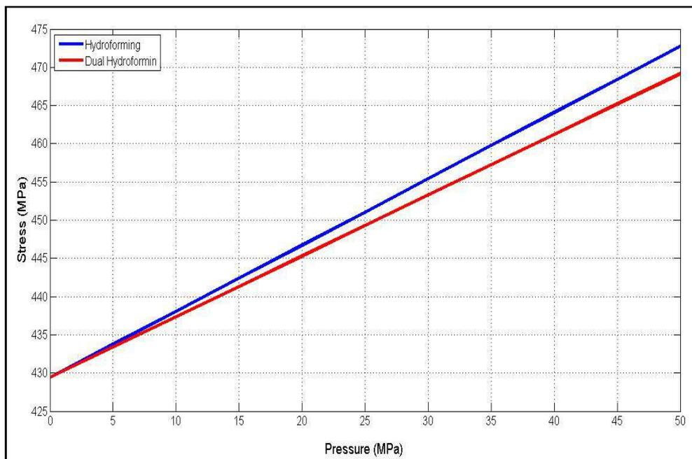
Figure13. The Applied Stress on the Deformation Zone
