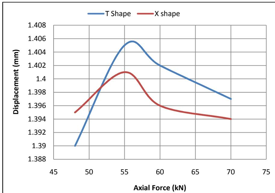
Figure8. The Effect of Changes in Axial Force Comparison in T-Shape and X-Shape in the Hydroforming Process
