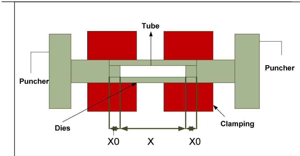
Figure1. The Schematic Model of a Tube Hydroforming System
