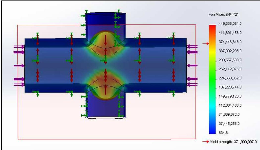
Figure5. Applied Stress in the X-Shape Tube Hydroforming, Inner Pressure 50 Mpa
