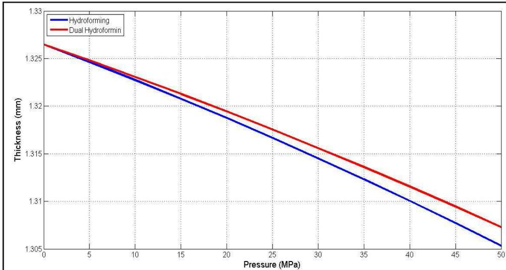
Figure12. The Changes of the Thickness through the Process
