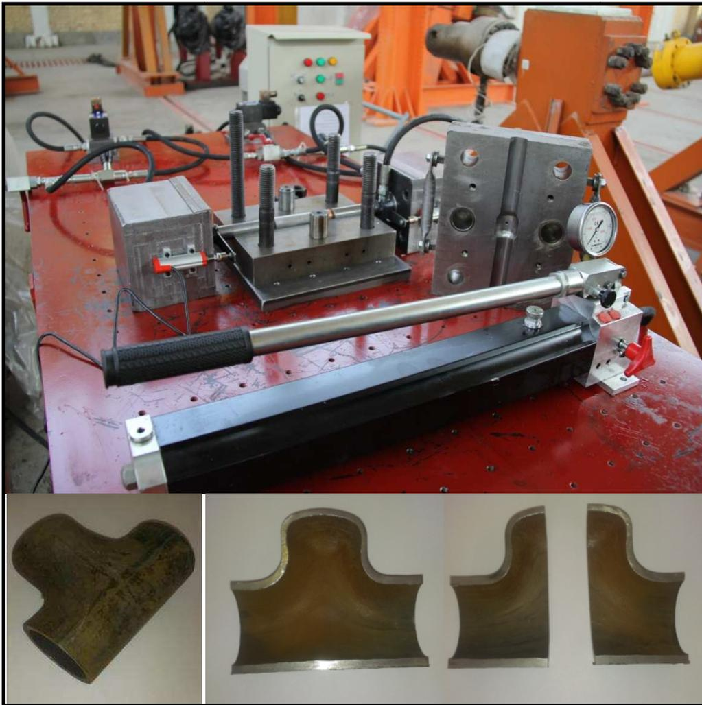
Figure11. The Developed Physical Hydroforming Machine
