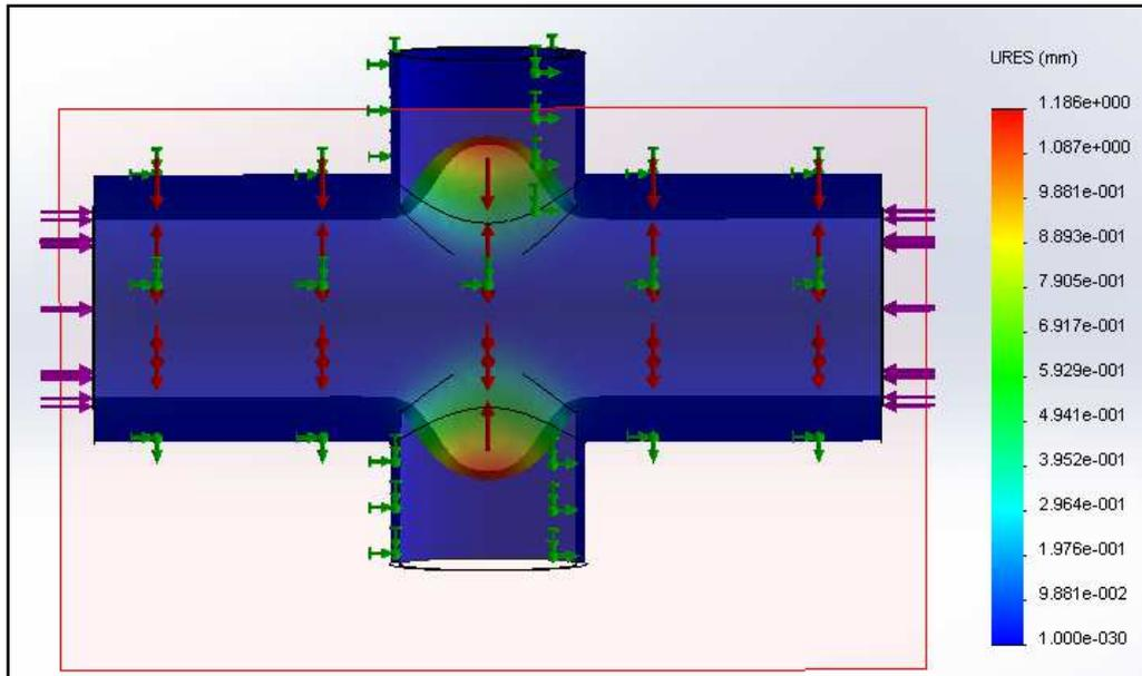
Figure6. Deformation in the X-Shape Tube Hydroforming, Inner Pressure 50 Mpa
