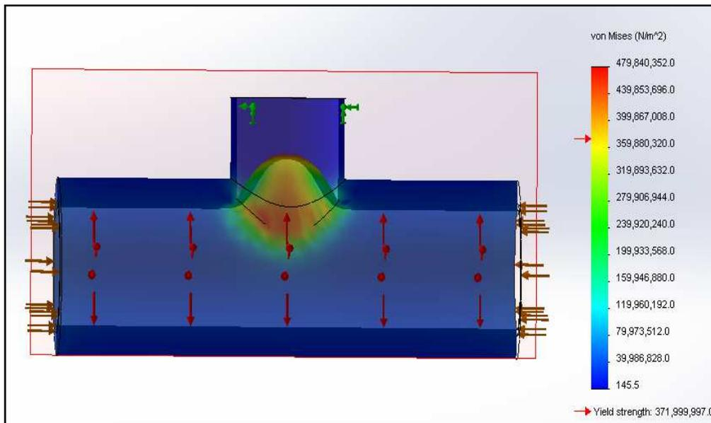
Figure3. Applied Stress in the T-Shape Tube Hydroforming, Inner Pressure 50 Mpa
