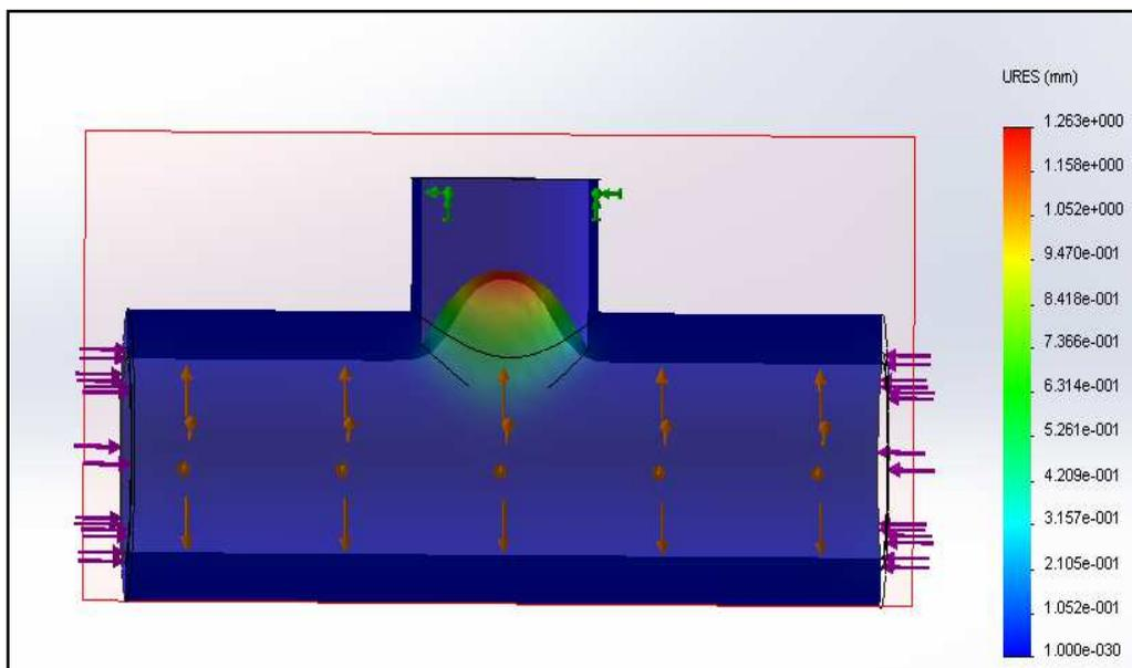
Figure4. Deformation in the T-Shape Tube Hydroforming, Inner Pressure 50 Mpa
