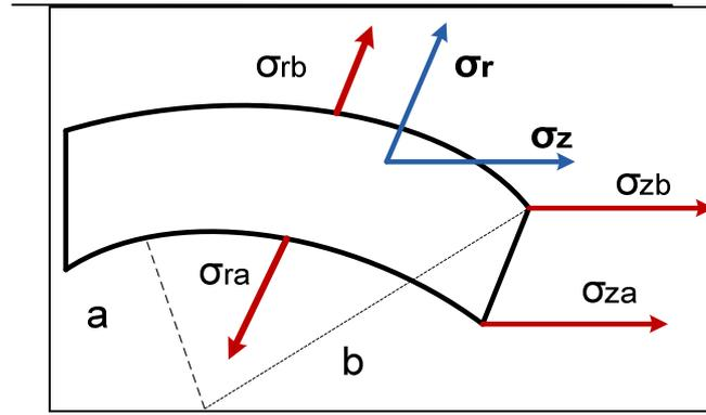
Figure2. The Applied Radial and the Axial Stress Diagram on the Tube
