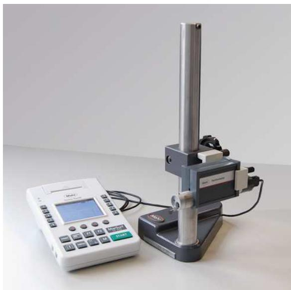
Figure2. The tool used for surface roughness measurement
