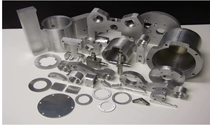
Figure5. Examples parts machined by water jet
