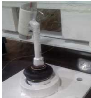
Figure9. Mechanism for setting injection angle
