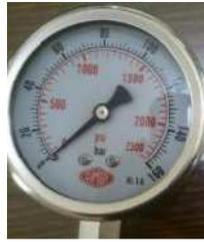
Figure19. Pressure gauge installed on system
