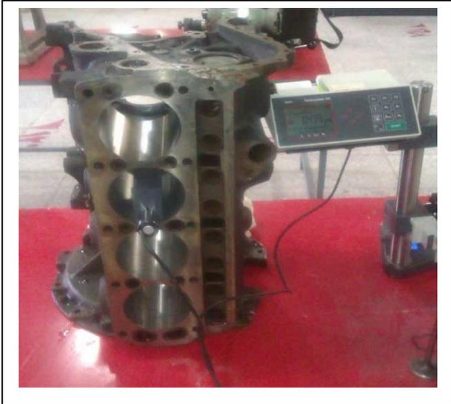
Figure4. Measuring surface roughness
