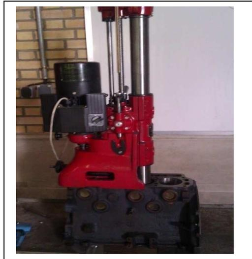
Figure2. Boring process
