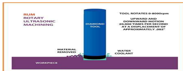
Figure4. Rotary ultrasonic machining process
