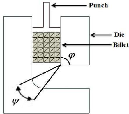
Figure 1. Schematic diagram of the ECAP die [41]
