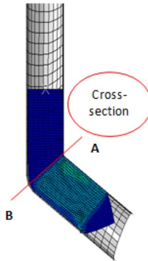
Figure 12. Die and the internal surface used for meshing
