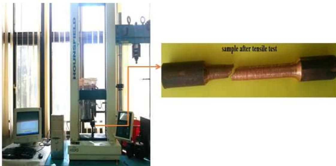
Figure 11. Tensile tester used in this study
